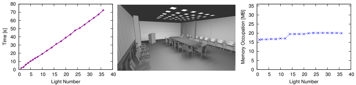
Figure 10: Increasing the number of lights. Left: The time consumption. Right: The maximum memory load reached during the computations. Center: A picture from our tests with 36 area light sources.
