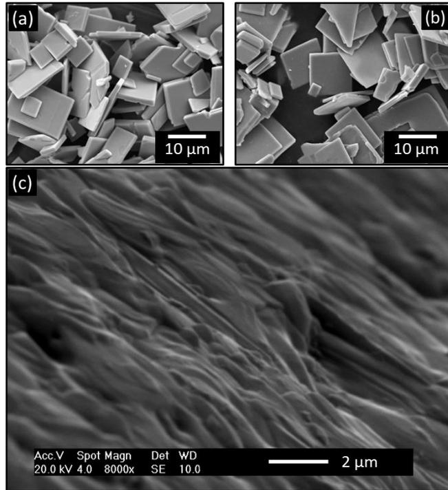
**Fig. 1:** SEM picture of (a) Bi<sub>2.5</sub>Na<sub>3.5</sub>Nb<sub>5</sub>O<sub>18</sub> platelets obtained by Molten Salts Synthesis, (b) NaNbO<sub>3</sub> templates obtained by Topochemical Conversion (c) BaTiO<sub>3</sub> – 8% volume NaNbO<sub>3</sub> textured sample (fracture).
