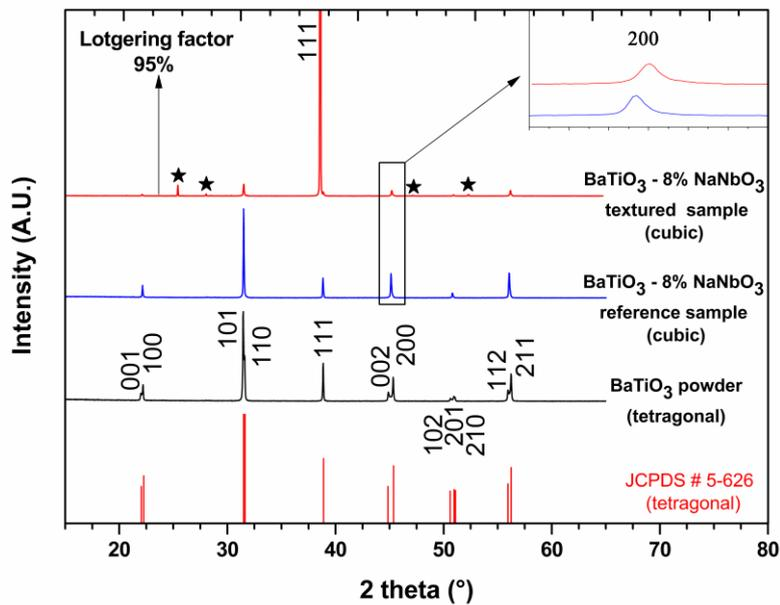
**Fig. 2:** X-ray diffraction patterns ( $\theta/2\theta$ , Cu  $K\alpha_1$ , color online): BaTiO<sub>3</sub> – 8% volume NaNbO<sub>3</sub> textured sample (stars = unidentified secondary phase), BaTiO<sub>3</sub> – 8% volume NaNbO<sub>3</sub> reference sample, tetragonal "pure" BaTiO<sub>3</sub> powder. Insert = detail showing the lack of splitting for (200) peak (the scale is different).
