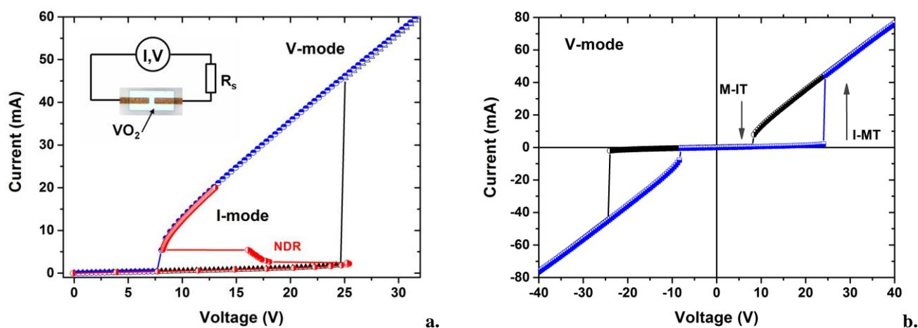
Figure 7. a. I-V characteristic in both V- and I-modes of a device incorporating a 20-  $\mu\text{m}$  length VO<sub>2</sub> pattern, with in insert, the electrical testing circuit; b. Current-voltage curves for the same device during positively and negatively sweeping of the applied voltage (V-mode operation) showing symmetrical behavior with respect to the origin of the I-V scale.
