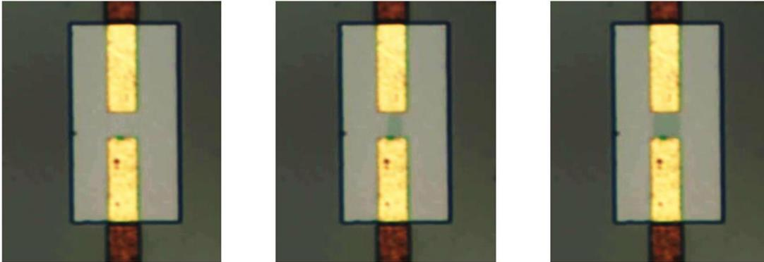
Figure 8. E-MIT inducing reflectivity changes of the VO<sub>2</sub> material, recorded in reflection-mode optical microscopy while the applied voltage on the electrodes of the 2T device is periodically swept between 0 and 40 V.
