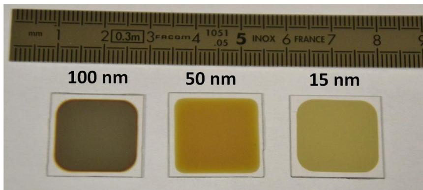
Figure 1. Photographs of typical VO<sub>2</sub> films with different thickness obtained by reactive electron-beam evaporation on 20x20 mm<sup>2</sup> sapphire substrates.
