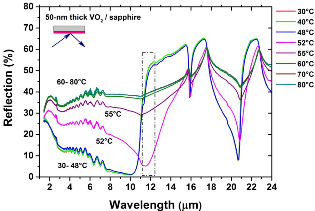
Figure 4. Temperature-dependent reflectivity curves for a 50-nm thick VO<sub>2</sub> layer on a sapphire substrate, obtained by FTIR spectroscopy.
