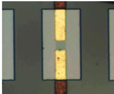
Video 1. Movie showing the periodical changes of the optical reflection of the VO<sub>2</sub>-based 2T device during periodical onset of the E-MIT in the VO<sub>2</sub> material (activation using a voltage waveform of 1 Hz and 40- V amplitude).
