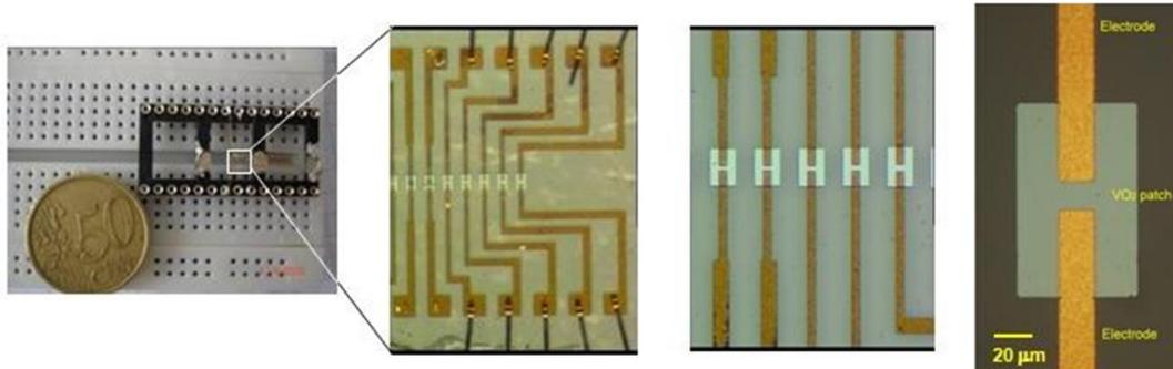
Figure 6. Photographs of typical fabricated two-terminal devices integrating VO<sub>2</sub> patterns obtained on sapphire substrates.
