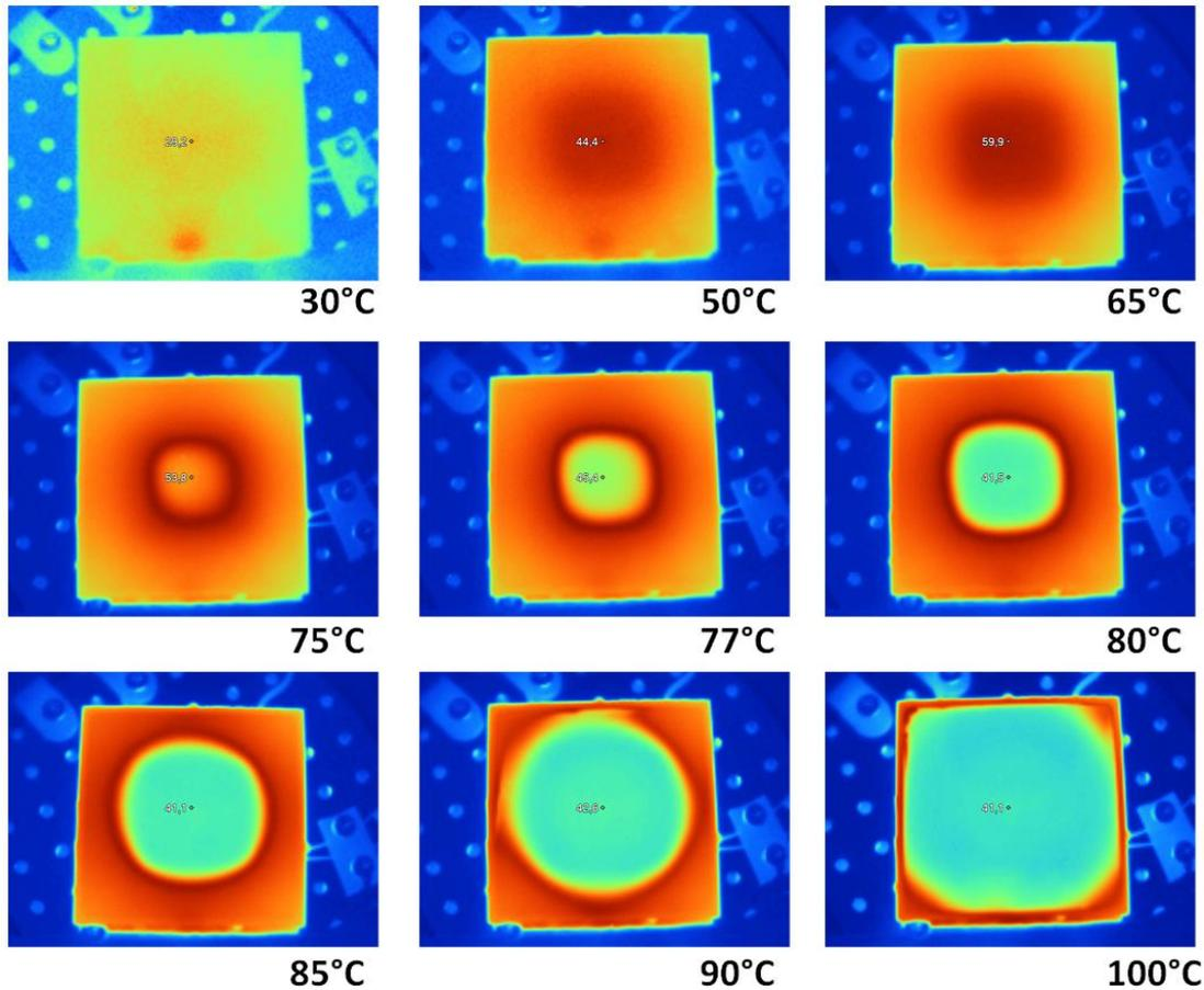
Figure 5. IR thermal images of a 50x50 mm<sup>2</sup> square 100-nm thick VO<sub>2</sub> layer on a sapphire substrate showing the phenomenon of negative differential emittance while heated across its MIT transition temperature.
