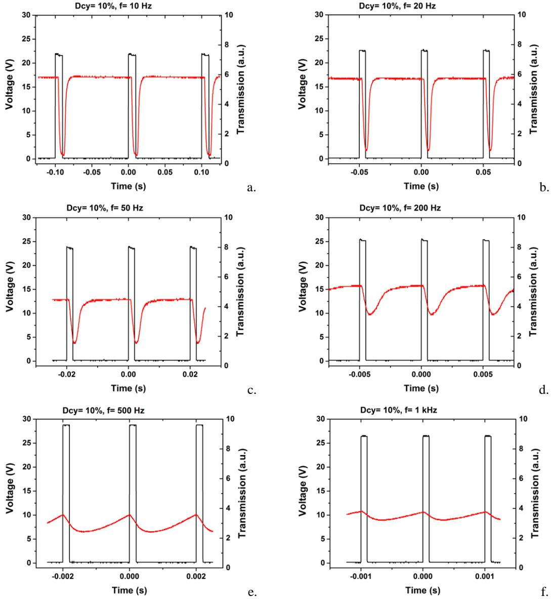
Figure 12. Frequency- dependent optical modulation variation of the VO<sub>2</sub>-based device when applying electrical pulses for a fixed DCy= 10% ( black curves: applied voltage pulses, red curves: optical transmitted power).
