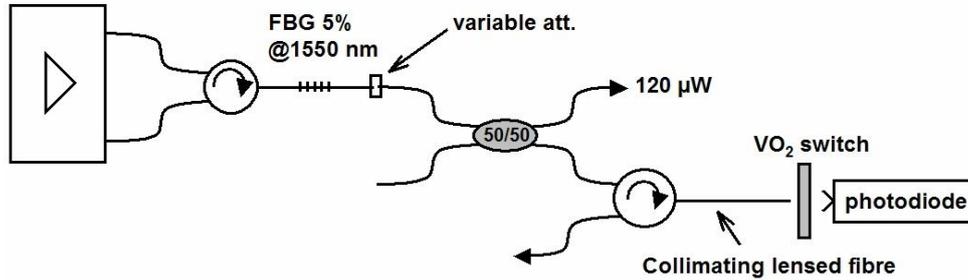
Figure 9. Experimental setup for the dynamical optical characterization (in transmission mode) of VO<sub>2</sub> patterns on sapphire substrates during electrical activation of their MIT.
