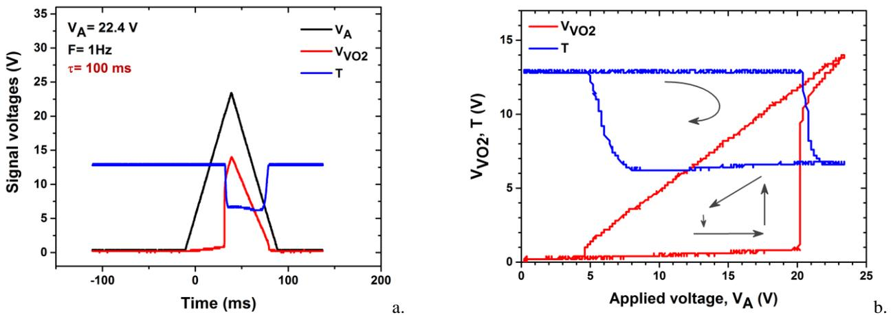
Figure 10. a. Dynamical optical transmission (at 1550 nm) of electrically activated VO<sub>2</sub> based optical device (black curve - applied voltage, blue curve - voltage drop across the DUT, blue curve - optical transmission), and b. the hysteresis of the electrical response and of the optical transmission of the device.
