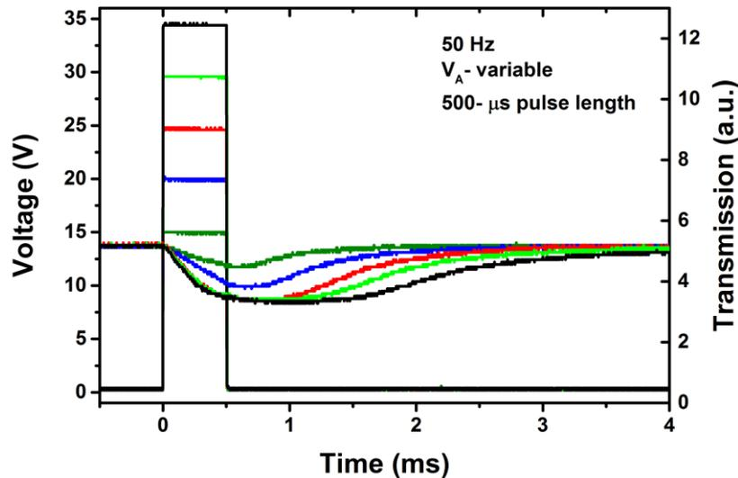
Figure 11. Temporal recordings of the optical transmission variation (dT) through the VO<sub>2</sub> device during the E-MIT through the application of corresponding square-type voltage pulses with different amplitudes.
