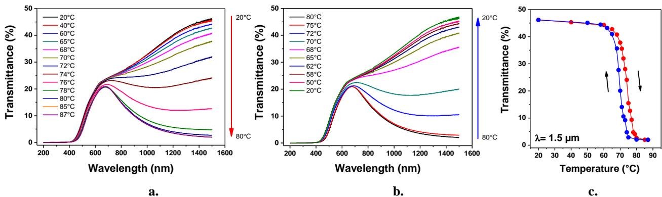
Figure 3. Temperature dependence of the optical transmission from 200 to 1600 nm for a 100-nm thick VO<sub>2</sub> films on sapphire: a. transmission variation for different temperatures during the heating cycle, b. the same recordings during the cooling cycle, c. hysteresis at  $\lambda = 1.5 \mu\text{m}$ .
