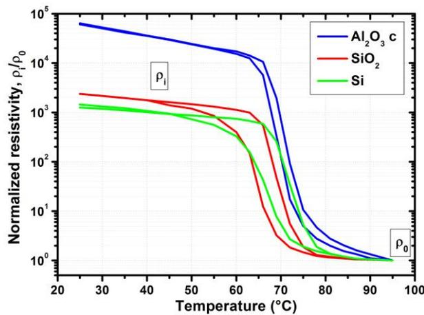
Figure 2. Typical electrical resistivity hysteresis curves (resistivity records during heating/cooling cycles) of VO<sub>2</sub> samples obtained on different substrates.
