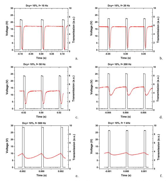
Figure 12. Frequency- dependent optical modulation variation of the  $VO_2$ -based device when applying electrical pulses for a fixed DCy=10% (black curves: applied voltage pulses, red curves: optical transmitted power).
