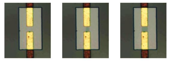
Figure 8. E-MIT inducing reflectivity changes of the VO2 material, recorded in reflection-mode optical microscopy while the applied voltage on the electrodes of the 2T device is periodically swept between 0 and 40 V.
