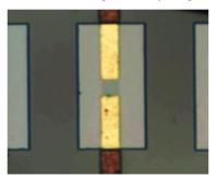
Video 1. Movie showing the periodical changes of the optical reflection of the VO<sub>2</sub>-based 2T device during periodical onset of the E-MIT in the VO2 material (activation using a voltage waveform of 1 Hz and 40- V amplitude). http://dx.doi.org/doi.number.goes.here
