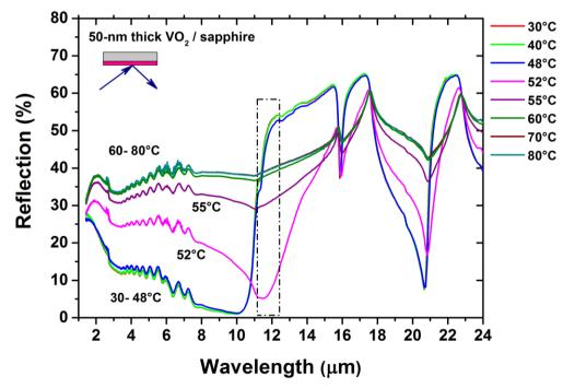
Figure 4. Temperature-dependent reflectivity curves for a 50-nm thick VO2 layer on a sapphire substrate, obtained by FTIR spectroscopy.
