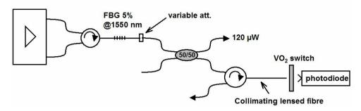
Figure 9. Experimental setup for the dynamical optical characterization (in transmission mode) of VO<sub>2</sub> patterns on sapphire substrates during electrical activation of their MIT.
