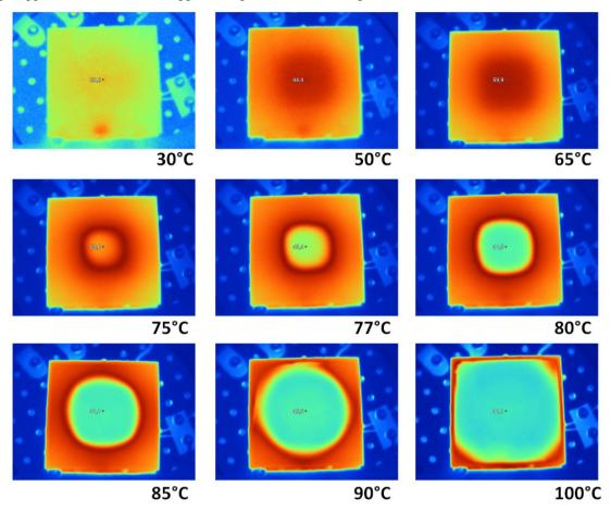
Figure 5. IR thermal images of a  $50x50 \text{ mm}^2$  square 100-nm thick VO<sub>2</sub> layer on a sapphire substrate showing the phenomenon of negative differential emittance while heated across its MIT transition temperature.
