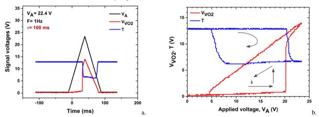
Figure 10. a. Dynamical optical transmission (at 1550 nm) of electrically activated VO2 based optical device (black curve - applied voltage, blue curve – voltage drop across the DUT, blue curve - optical transmission), and b. the hysteresis of the electrical response and of the optical transmission of the device.
