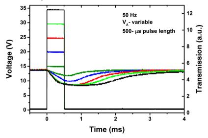
Figure 11. Temporal recordings of the optical transmission variation (dT) through the VO2 device during the E-MIT through the application of corresponding square-type voltage pulses with different amplitudes.
