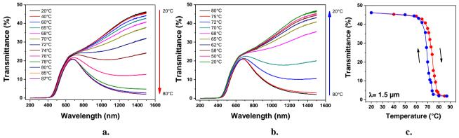
Figure 3. Temperature dependence of the optical transmission from 200 to 1600 nm for a 100-nm thick VO2 films on sapphire: a. transmission variation for different temperatures during the heating cycle, b. the same recordings during the
