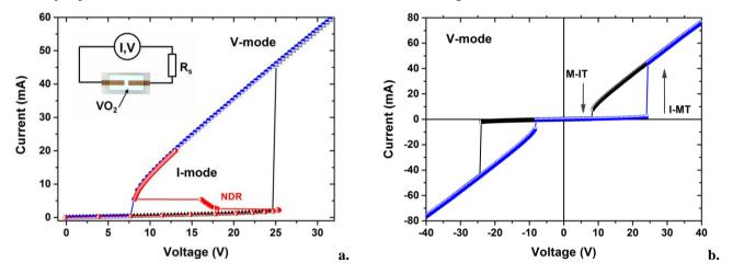
Figure 7. a. I-V characteristic in both V- and I-modes of a device incorporating a 20- μm length VO2 pattern, with in insert, the electrical testing circuit; b. Current-voltage curves for the same device during positively and negatively sweeping of the applied voltage (V-mode operation) showing symmetrical behavior with respect to the origin of the I-V scale.
