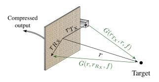
Fig. 3: Metamaterial aperture made of coupled cELC unit cells, associated with a radiating horn.
