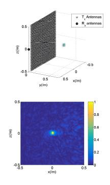
Fig. 5: 3D point spread function for pseudo-inversion of the compressive device radiation discretized on a set of voxels and 2D extraction from the y = 0.5m plane
