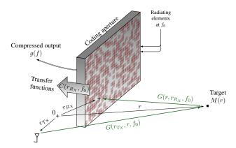
Fig. 1: Imaging system composed of a transmitting antenna and a receiving compressive aperture.
