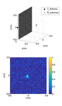
Fig. 4: 3D point spread function for a reconstruction of aperture's field and a range migration algorithm and 2D extraction from the y = 0.5m plane
