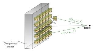
Fig. 2: Illustration of a passive multiplexer connected to an array of UWB Vivaldi antennas.
