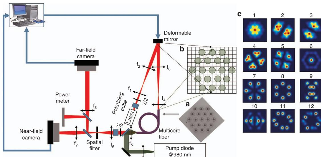
**Figure 1** Schematic of the experimental setup including (a) an image of the MM-MC Yb-fiber (in gray), (b) a drawing of the downscale imaging of the DM surface on the fiber input face and (c) the 12 supermode patterns.
