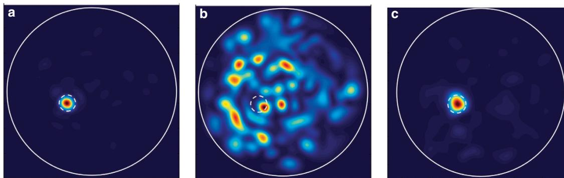
**Figure 8** Highly multimode fiber amplifier, experimental output patterns (a) after adaptive structuring of the input wavefront to obtain maximum power in the small target area bounded by the white dotted line without gain; (b) after switching on the gain, while maintaining the mirror profile with the passive case setting; and (c) after a restart of the adaptive profiling for shaping with a gain of  $\sim 20$  dB.
