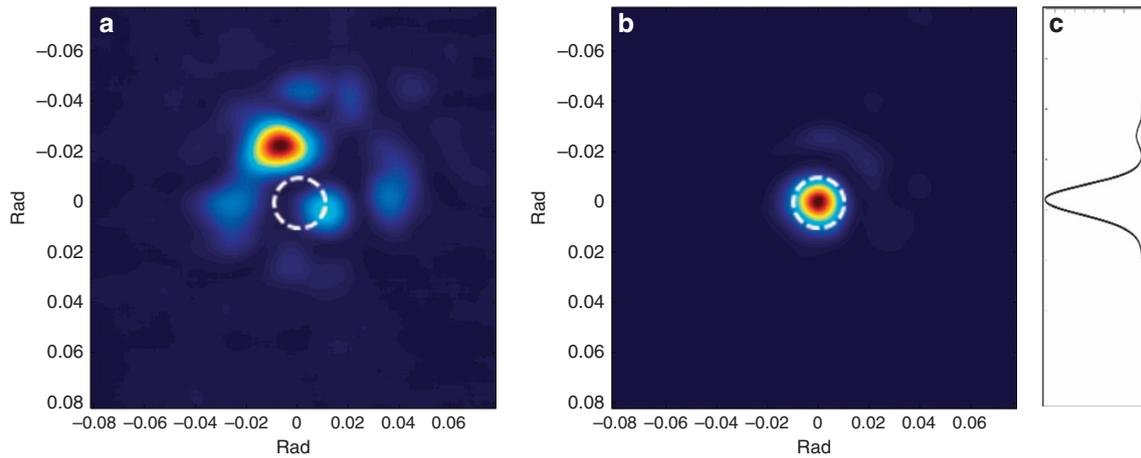
**Figure 6** Experimental far-field pattern of the multicore fiber amplifier before wavefront shaping (a), final pattern after optimization of the DM surface to obtain, in the desired orientation (dashed white circle), a single narrow diffraction lobe (b) and cross-sectional profile (c).
