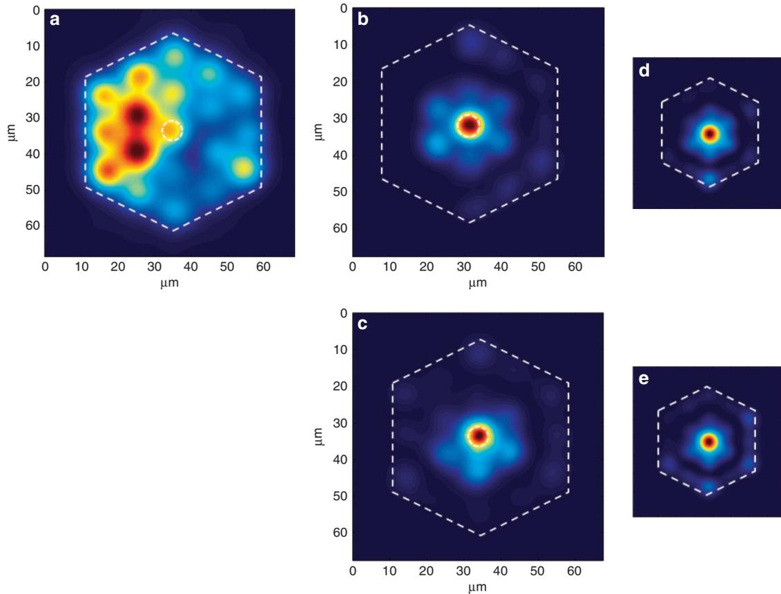
**Figure 2** Output patterns recorded on the exit face of the MM-MC Yb-doped optical fiber: (a) without wavefront profiling, (b) after wavefront shaping for focusing on the central core without gain and (c) after wavefront shaping with 17-dB small signal gain. Insets show numerical results of the modeling of the whole system for the passive (d) and active (e) regimes, in good agreement with the observations.
