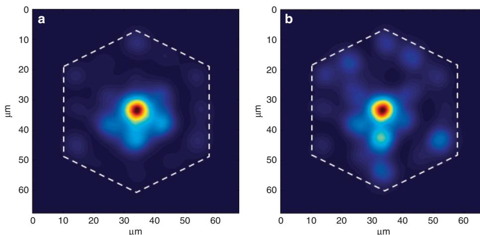
**Figure 5** Comparison of the pattern recorded at the amplifier output for (a) the small signal amplification regime and for (b) amplification in the saturation regime ( $-6$  dB gain drop) with concentration of the amplified light on a central spot.
