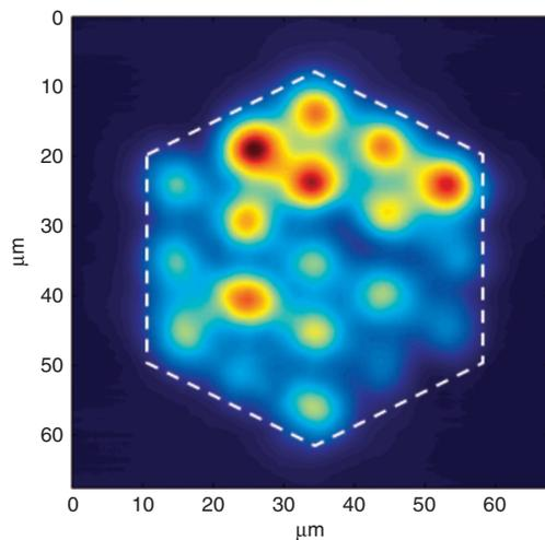
**Figure 7** Near-field intensity at the MM fiber amplifier output recorded after optimization in the far field corresponding to Figure 6b. Clearly, the pattern does not correspond to the fundamental mode profile of the structure.
