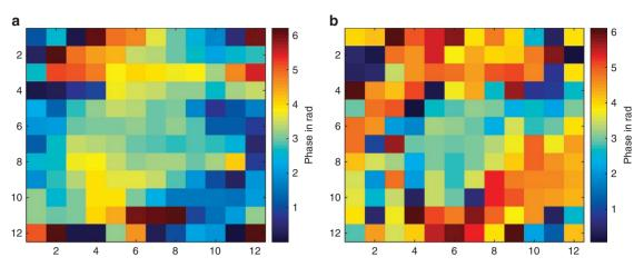
Figure 3 Experimental phase pattern imprinted on the Gaussian laser beam at the input to obtain a single bright spot on the MM fiber output without (a) and with (b) gain (unsaturated).
