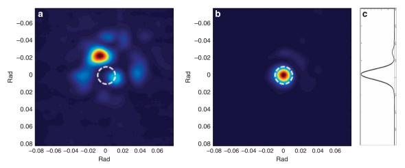
Figure 6 Experimental far-field pattern of the multicore fiber amplifier before wavefront shaping (a), final pattern after optimization of the DM surface to obtain, in the desired orientation (dashed white circle), a single narrow diffraction lobe (b) and cross-sectional profile (c).
