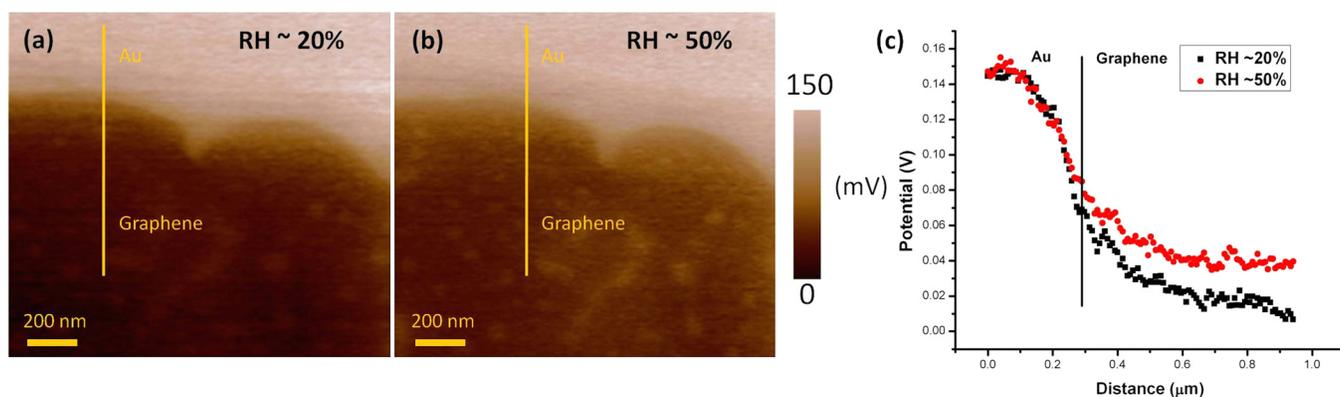
FIG. 6. SKPM images of functionalized graphene at different humidity levels: (a) RH  $\sim$  20%; (b) RH  $\sim$  50%. (c) The graph shows the potential variations corresponding to the same selected location marked with the yellow line in (a) and (b) for RH  $\sim$  20% (black) and RH  $\sim$  50% (red).
