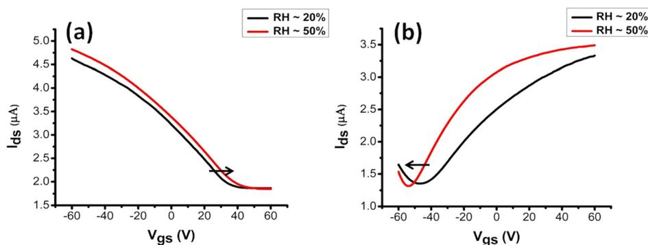
FIG. 7. Transfer curves under  $V_{ds} = 10$  mV for (a) non-functionalized and (b) PEI-functionalized graphene at different humidity levels: RH  $\sim$  20% (black) and RH  $\sim$  50% (red).
