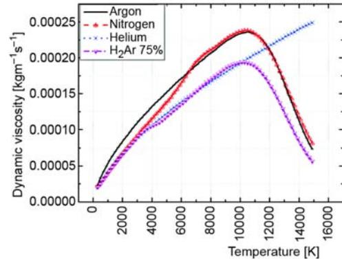
**Figure 4. Atmospheric pressure dynamic viscosity of pure gases Ar, He, N<sub>2</sub> and the mixture H<sub>2</sub>Ar75%**
