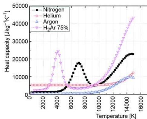
**Figure 2. Specific heat capacity of pure gases Ar, He, N<sub>2</sub> and the mixture H<sub>2</sub>Ar75% at atmospheric pressure**
