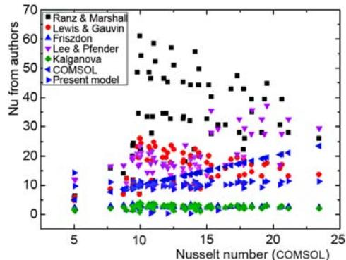
**Figure 11.** Nusselt number correlations as a function of  $\text{Nu}_C$  for  $\text{H}_2\text{Ar}75\%$
