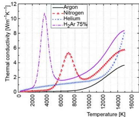
**Figure 3. Thermal conductivity of pure gases Ar, He, N<sub>2</sub> and the mixture H<sub>2</sub>Ar75% at atmospheric pressure**
