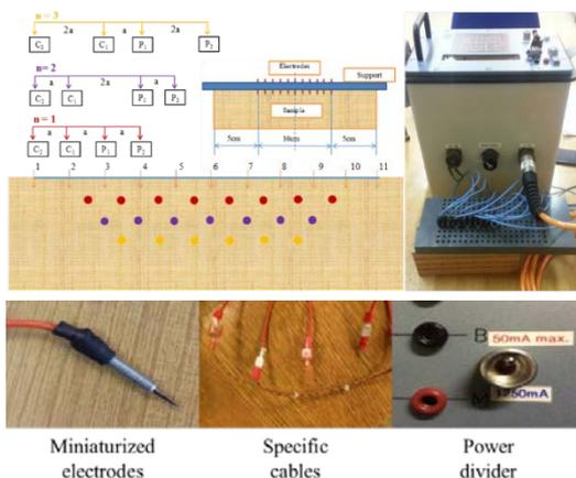
**Figure 1.** Distribution of electrodes and 3 dipole-dipole levels.
