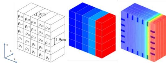
Figure 4. Discretization of sample, resistivity field projection.
