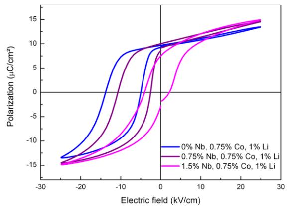
Fig. 2. P-E hysteresis loops of  $\text{BaTiO}_3$  doped with  $\text{Co}^{2+/3+}$  and different amount of  $\text{Nb}^{5+}$ .
