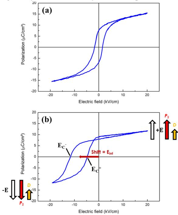
Fig. 1. P-E hysteresis loops of (a) pure  $\text{BaTiO}_3$  (typical hysteresis loop) and (b) poled  $\text{Co}^{2+/3+}$ -doped  $\text{BaTiO}_3$  with a representation of the ferroelectric domains and defect dipoles orientation depending on the applied electric field.
