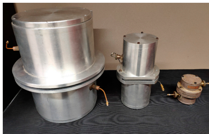
Figure 3. The resonant cavities used for dielectric characterization for Epson paper.
