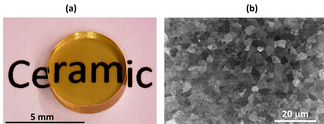
Figure 1. (a) Picture taken of a typical bulk tellurite ceramic, placed above a text, and dedicated for performing laser emission tests. (b) SEM observation of the polished surface, revealing the ceramic grains (please note that the contrast of the picture was enhanced and that no chemical etching was used).
