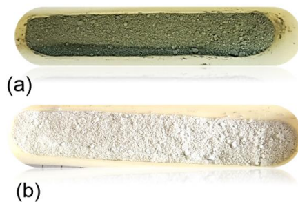
Figure S2 Aspect of a typical \text{TiO}_2 /graphene nanopowder obtained by laser pyrolysis before (a) and after (b) thermal annealing at 430^\circ\text{C} for 6h in air.
