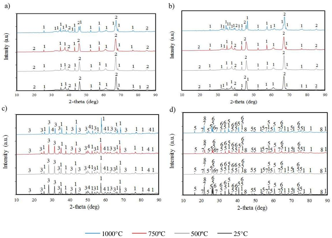
1. Al<sub>2</sub>O<sub>3</sub>-α    2- Al<sub>2</sub>O<sub>3</sub>-γ    3. ZrO<sub>2</sub>-m    4. ZrO<sub>2</sub>-c    5. Mullite    6. Sillimanite
