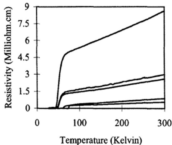
**Figure 1 :** Typical resistivity versus temperature for different films obtained with various sequences of pulses. The film in which  $\text{O}_8$  phase has been identified shows the lowest resistivity at 300 K.
