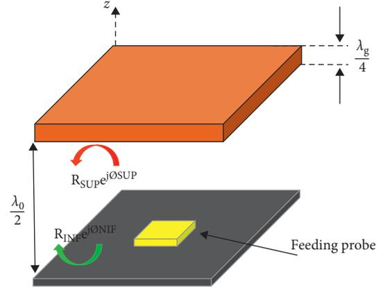
FIGURE 1: Classical EBG antenna fed by a patch.
