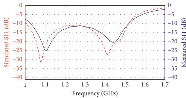
FIGURE 10: Theoretical and experimental  $S_{11}$  evolution vs frequency.
