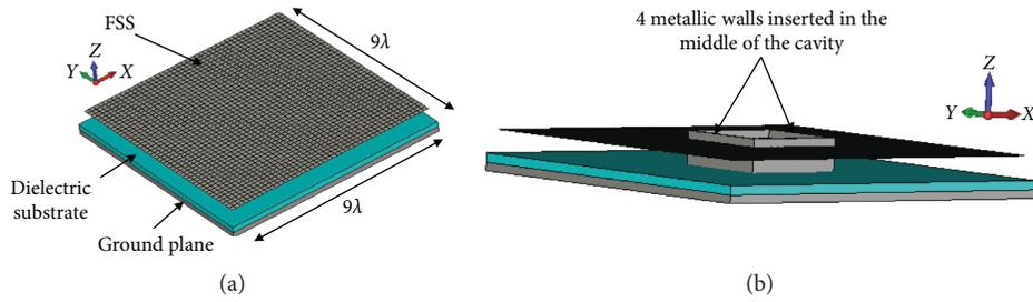
FIGURE 2: (a) High-gain EBG Antenna. (b) Vertical metallic walls inside the EBG antenna.
