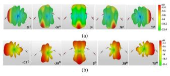
Figure 8. Beam-steering situations of the selected phased array, (a) Far-field radiation patterns, (b) Near-field radiation pattern.
