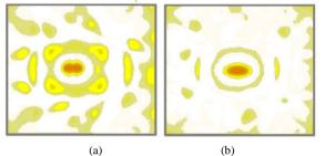
Figure 10. Imaging result for two targets with 1 cm horizental distance between them achieved by (a) the rectangular antenna array, and (b) the round antenna array.
