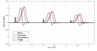
Figure 7. The reflected waveforms comparison for simulated results by ADS, idael pulse, Gaussian, Lorentzian and Voigt pulses for the biological tissue phantom with a target.
