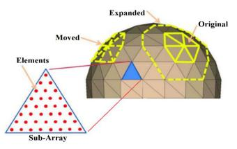
Figure 3. Scheme of the envisioned cognitive partitioning of sub-arrays in the proposed HMPAR framework.
