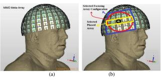
Figure 5. (a) Meta-array of the MIMO array for signalling strategies, and (b) Sub-array selection for beemsteering and beamforming (balck: refrence transmitter in focusing algorithm, red: round array configuration, blue: rectangular array configuration and yellow: phased array configuration).
