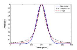
Figure 6. Graph of the Gaussian, Lorentzian and Voigt (their convolution) functions.
