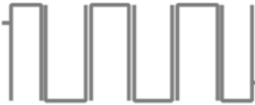
Figure 4.7 – Layout of the classical Chebyshev filter implemented as aligned hairpin coupled resonators. Reprinted with permission from ref. [1]; copyright 2014 IEEE.
