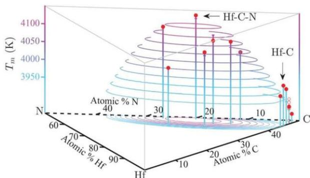
Figure 4. Melting temperatures of materials compositions in the Hf-C-N and Hf-C (red filled circles) as well as Hf-Ta-C (empty circles) systems (Reproduced with permission.<sup>[77]</sup> Copyright, American Physical Society).
