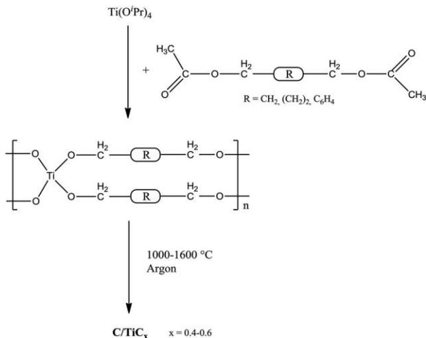
Figure 7. Schematic description of the synthesis of TiC from polymeric titanates.<sup>[109]</sup>
