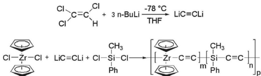
Figure 19. Synthesis of a Zr and Si containing poly-yne polymer used as a single-source precursor for the synthesis of ZrC/SiC nanocomposites.<sup>[193]</sup>
