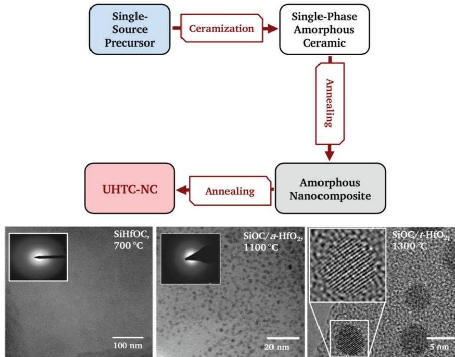
Figure 5. Typical preparative approach of polymer-derived ceramic nanocomposites starting from single-source precursors.<sup>[87–89]</sup>
