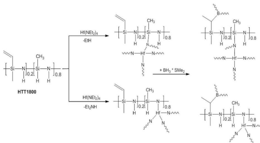
Figure 22. Modification of HTT1800 with Hf(NEt<sub>2</sub>)<sub>4</sub> and BH<sub>3</sub>·SMe<sub>2</sub> (Reproduced with permission.<sup>[202]</sup> Copyright, ACS, 2014)
