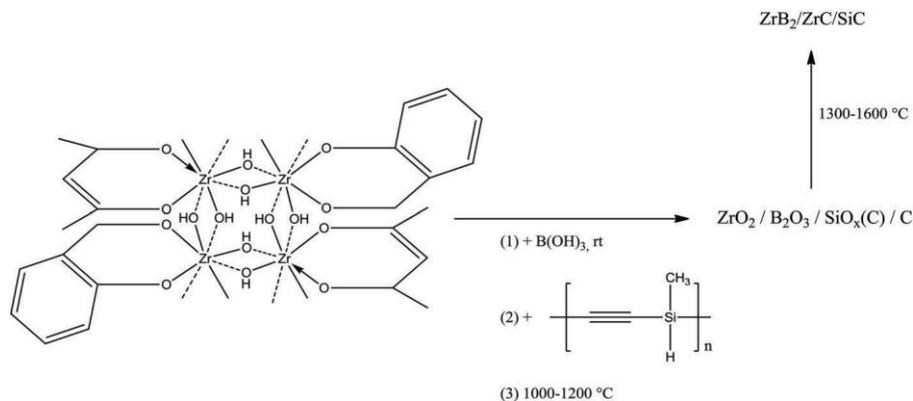
Figure 12. Synthesis of ZrB<sub>2</sub>/ZrC/SiC from a polymer blend consisting of B(OH)<sub>3</sub>-modified polyzirconoxanesal and poly(methylsilylene-ethynylene) upon high-temperature thermal treatment in argon atmosphere.<sup>[141]</sup>
