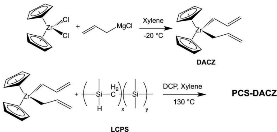
Figure 17. Synthesis of DACZ and reaction with a low molecular weight PCS.<sup>[183]</sup>
