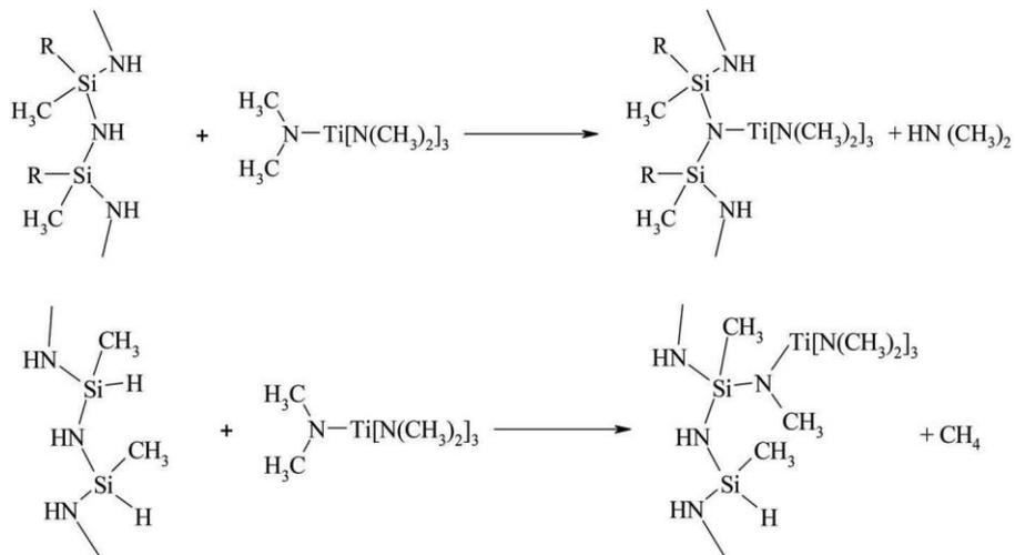
Figure 14. Reaction between NH and SiH units present in polysilazanes and NCH<sub>3</sub> groups present in TDMATi.<sup>[154]</sup>
