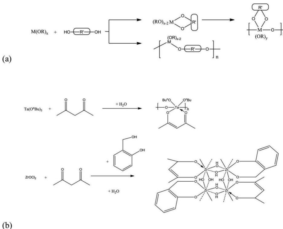
Figure 8. Synthetic access to polymeric metallates; a) based on metal alkoxides and di-alcohols  $\text{R}'$  alkyl;  $\text{R}' = \text{C}_x\text{H}_{2x}$ <sup>[113,121]</sup>; (b) based on metal alkoxides and acetylacetone<sup>[118]</sup> as well as on metal salts and a combination of acetylacetone and a di-alcohol.<sup>[117]</sup>
