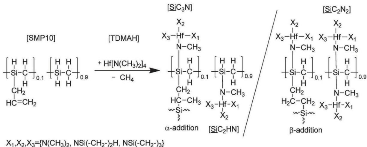
Figure 18. Modification of AHPCS with  $Hf(NEt_2)_4$  leading to two silicon environments in the resulting preceramic polymer (Reproduced with permission<sup>[187]</sup>; we acknowledge the Royal Society of Chemistry for the reproduced material).
