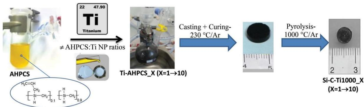
Figure 15. Overall process for preparing dense monolithic Si–C–Ti components.<sup>[165]</sup>
