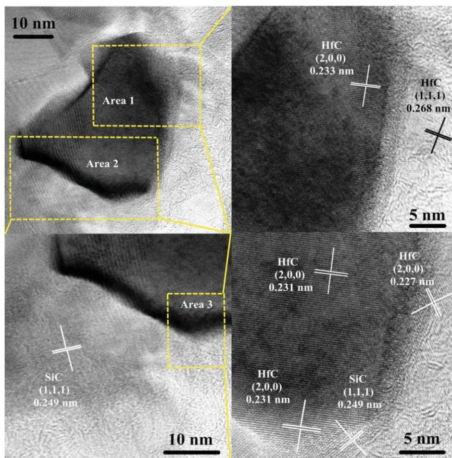
Figure 16. TEM images of polymer-derived HfC/SiC powders at  $1600^\circ\text{C}$ <sup>[139]</sup> (reprinted with permission from Wiley, 2018).
