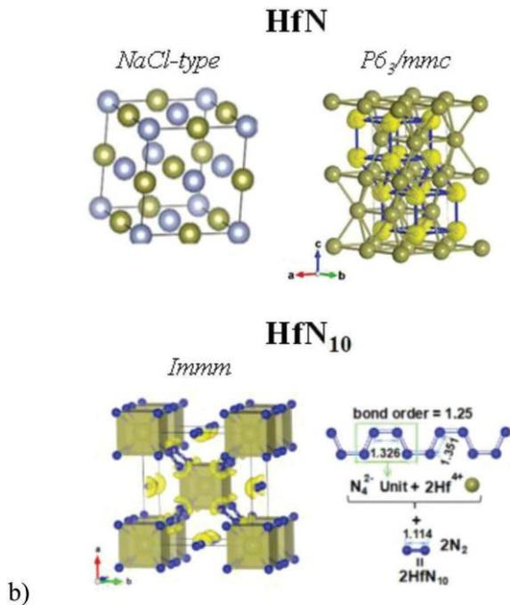
Figure 2. a) Phase diagram of the Hf–N system (Reproduced with permission.<sup>[65]</sup> Copyright, Springer); b) crystalline structures of HfN (*NaCl*-type and *P6<sub>3</sub>/mmc*) and of HfN<sub>10</sub> (*Immm*). For *Immm*-HfN<sub>10</sub>, infinite polymeric nitrogen chains and N<sub>2</sub>-N bondings are shown (Reproduced with permission.<sup>[67]</sup> Copyright, American Physical Society).
