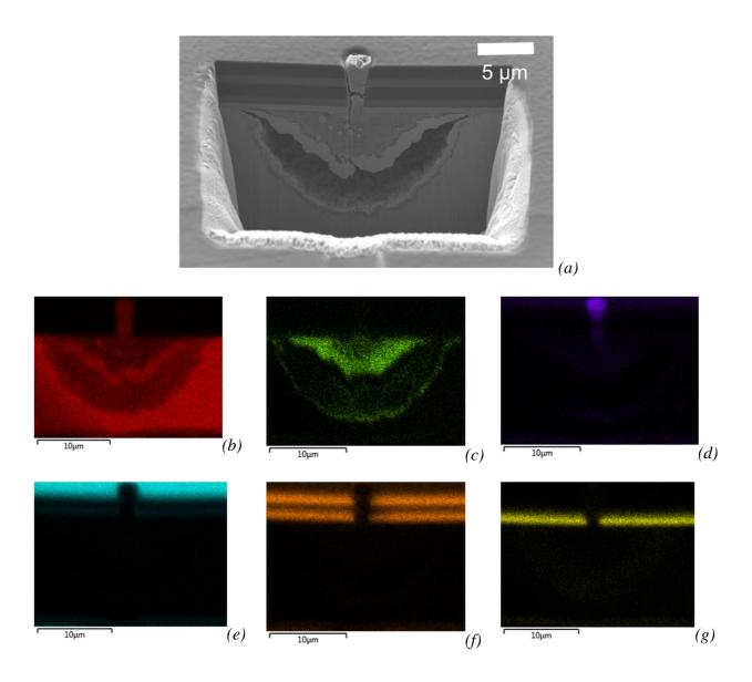
Figure 10- SEM observation and chemical composition map analysis of a cross-section obtained on a 2.5  $\mu$ m diameter artificial defect produced using FIB and after "in situ electrochemical test"
