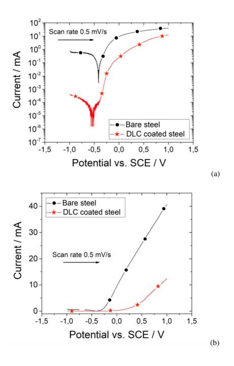
Figure 4 - Polarization curves for a bare and coated with DLC 100Cr6 steel plotted in logarithm current scale (a) and in linear current scale (b)
