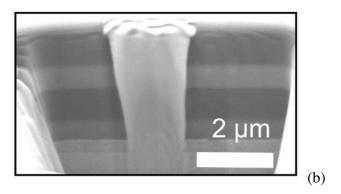
*Figure 7-* SEM top surface(a) and cross-sectional (b) views of a 2.5  $\mu$ m diameter artificial defect produced by FIB machining.
