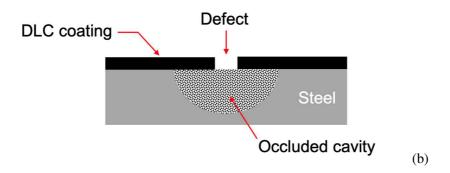
Figure 9 – Characteristics of an artificial propagating defect
