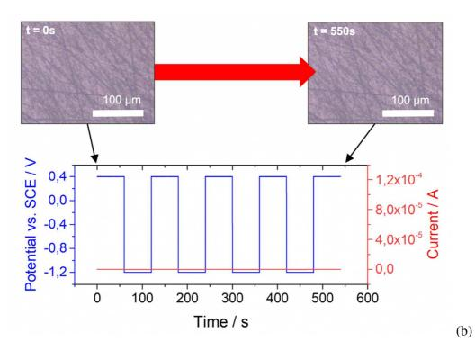
**Figure 6** – In situ temporal series of microscope imaging coupled with electrochemical activation induced by a pulse sequence cycling the potential from a cathodic (1 min) to an anodic (1 min) value.
