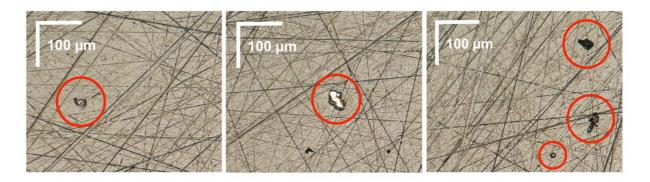
Figure 2- Typical defects due to the presence of dusts particles (substrate roughness Ra = 0.05  $\mu m$ )
