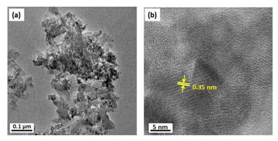
Fig. 5. Transmission electron micrograph illustrating (a) uniform distribution of the  $TiO_xN_y$ -derived materials and (b) Lattice fringes unveiling a spacing of 0.35 nm consigned to (1 0 1) plane of the anatase phase in the  $TiO_xN_y$ -derived materials.
