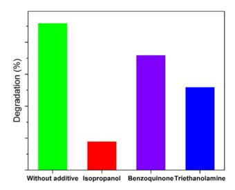
Fig. 12. . Catalytic degradation efficiency of methylene blue solution with and without the presence of presence of scavengers.
