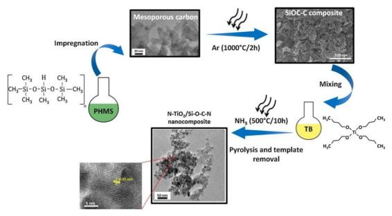
Fig. 1. Schematic representing the generalized processing route for the synthesis of the mesoporous nanocomposite.
