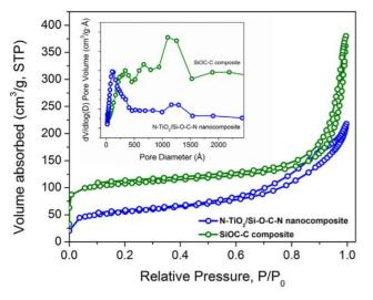
Fig. 6.  $N_2$  adsorption-desorption isotherm indicating the presence of mesopores in SiOC-C composite and N-TiO<sub>2</sub>/Si-O-C-N nanocomposite and the inset image shows the BJH pore size distribution curve.
