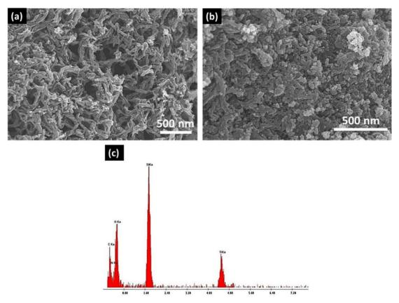
Fig. 4. Scanning electron micrograph exhibiting the porous nature of (a) CMK-3 (b) the TiO<sub>x</sub>N<sub>y</sub> derived materials and (c) EDS spectrum of the nanocomposite.
