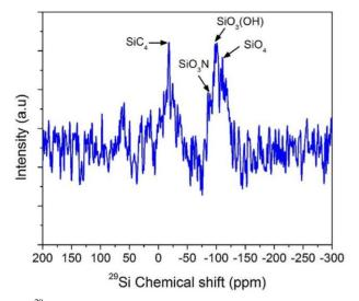
Fig. 9. <sup>29</sup>Si MAS NMR spectra of N-TiO<sub>2</sub>/Si-O-C-N nanocomposite implying the incorporation of N atoms in the Si-based network.
