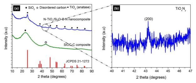
Fig. 2. (a) X-ray diffractrograms revealing the amorphous and crystalline phases of the nanocomposite before and after functionalization with TB and (b) The slow scan XRD of N-TiO<sub>2</sub>/Si-O-C-N exemplifying the TiO<sub>3</sub>N<sub>y</sub> phase.
