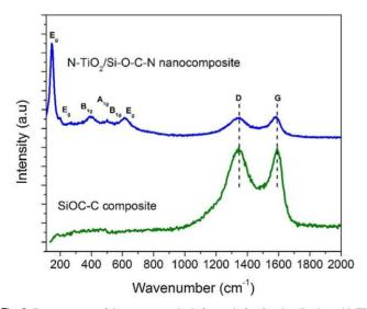
Fig. 3. Raman spectra of the nanocomposite before and after functionalization with TB implying the presence of anatase phase and free carbon.
