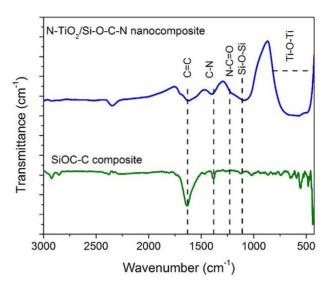
Fig. 8. FTIR spectrum showing the bonding characteristics of the SiOC-C composite and N-TiO $_2$ /Si-O-C-N nanocomposite.
