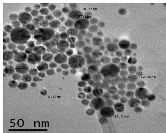
**Figure 2: TEM images of gold nanoparticles (AuNP@PEI) with ratio (m<sub>PEI</sub>/m<sub>Au</sub> = 0.46)**
