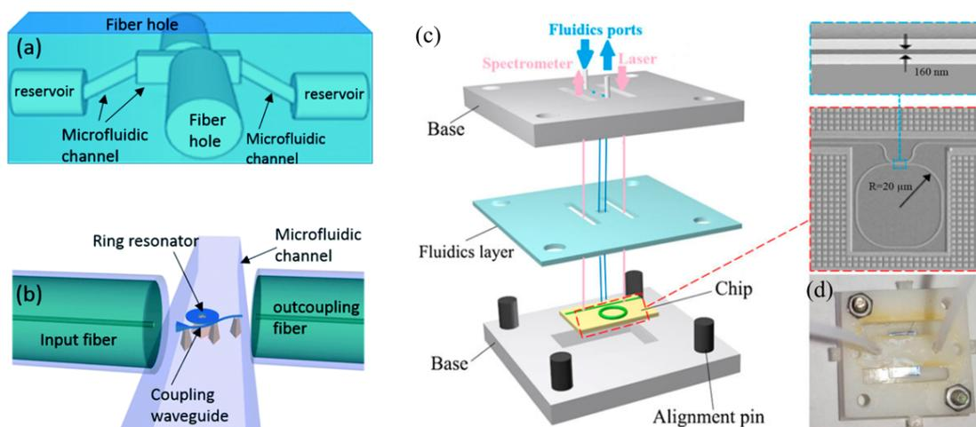
**Figure 4.** On-chip planar resonators for sensing. (a) Schematic view of the glass microfluidic chip; (b) detail of the WGM biosensor integrated inside the microfluidic channel. Reproduced from ref. <sup>[104]</sup> with permission of Royal Society of Chemistry. (c) Schematic illustration of the integrated sensing system. (d) Photograph of the PDMS microfluidic channels. Reproduced from ref. <sup>[105]</sup> with permission of AIP Publishing.
