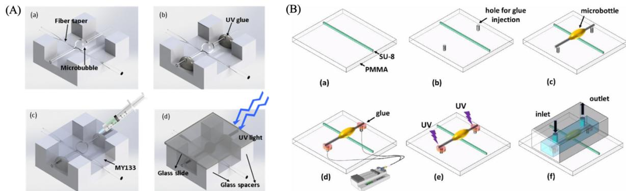
**Figure 8.** (A) Packaging process of microbubble resonators. Reproduced from ref. <sup>[166]</sup> with permission of Optical Society of America. (B) Lab-on-chip platform fabrication and packaging steps of microbottle resonators. Reproduced from ref. <sup>[167]</sup> with permission of Elsevier.
