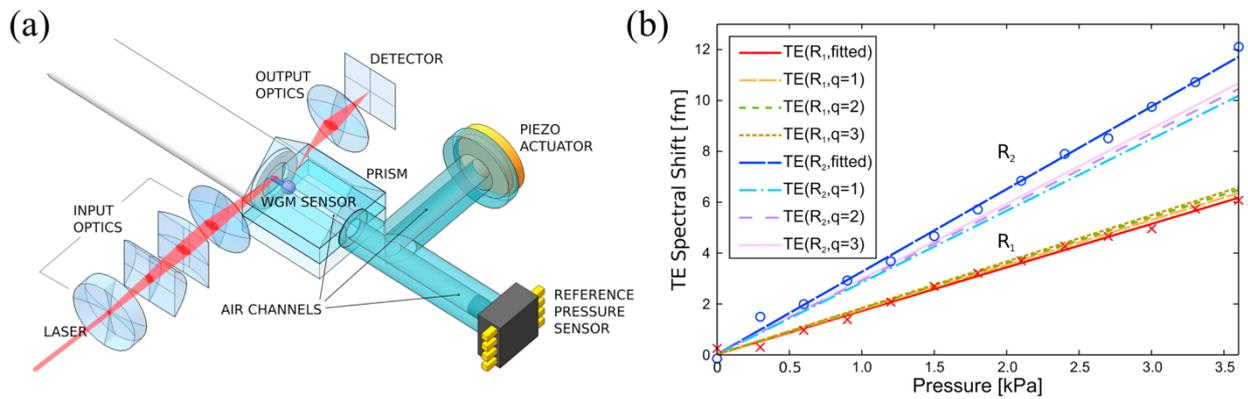
**Figure 13.** (a) Experimental setup of the WGM pressure sensing platform. (b) Spectral shift versus pressure for two spheres of radii  $R_1=127\ \mu\text{m}$  and  $R_2=89\ \mu\text{m}$ . Reproduced from ref. <sup>[213]</sup> with permission of Elsevier.
