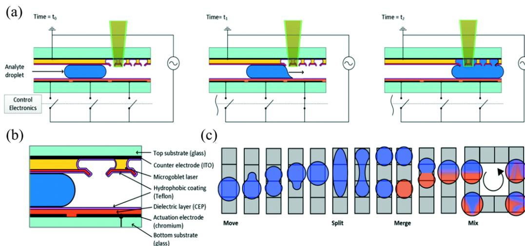
**Figure 6.** Cross-sectional view of a digital microfluidic system integrated with microgoblet resonators. (a) Analyte delivery process through activating the electrodes. (b) Close-up of the integrated system depicting the material layers (c) Some basic on-chip microfluidic operations. Reproduced from ref. <sup>[134]</sup> with permission of Royal Society of Chemistry.
