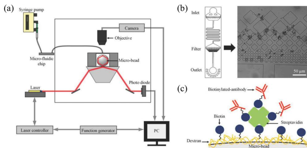
**Figure 10.** Microfluidic integrated WGMB. (a) WGMB system schematic. (b) Left: Microfluidic chip. Right: The Jurkat cells trapped in the microfluidic device. (c) Illustration of surface functionalization. Reproduced from ref. <sup>[191]</sup> with permission of John Wiley and Sons.
