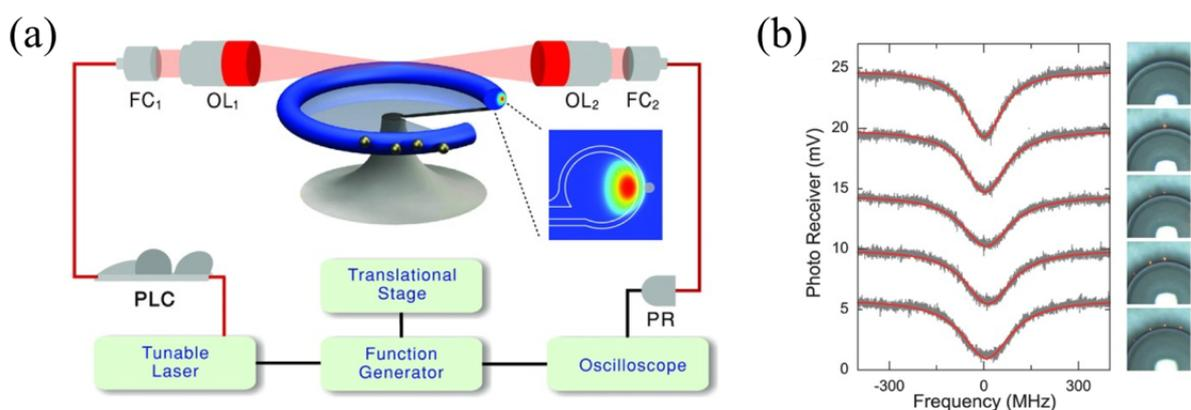
**Figure 2.** Mode-broadening based sensing (a) Experimental setup for mode-broadening based PS nanoparticles and virus detection. (b) Transmission spectra of the mode and the corresponding microcavity-enhanced-scattering optical images upon binding of 0 - 4 nanoparticles (from top to bottom). Reproduced from ref. [25]. Copyright 2013 John Wiley and Sons.
