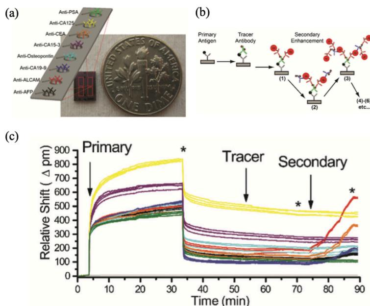
**Figure 9.** (a) Silicon microchip overlaid with four red boxes indicating sub-array regions containing 8 microring resonators, each functionalized with an antibody specific for a different cancer biomarker antigen. (b) Methodology of the layer-by-layer signal enhancement on the microring resonator silicon surface. (d) A real-time plot showing the resonance wavelength shifts through the entire bioassay. Reproduced from ref. <sup>[189]</sup> with permission of Royal Society of Chemistry.
