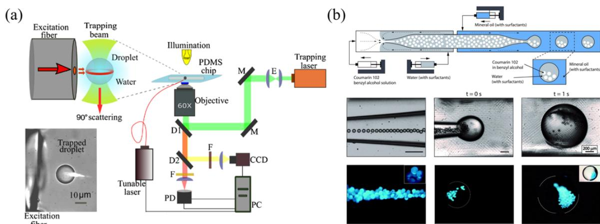
**Figure 7.** (a) Experimental setup of microdroplet scattering experiments and an image of scattered light when the trapped droplet was excited by a red laser. Reproduced from ref. <sup>[145]</sup> with permission of The Optical Society. (b) Glass capillary devices to embed liquid lasers within aqueous microfluidic droplets. Reproduced from ref. <sup>[148]</sup> with permission of Wiley Online Library.
