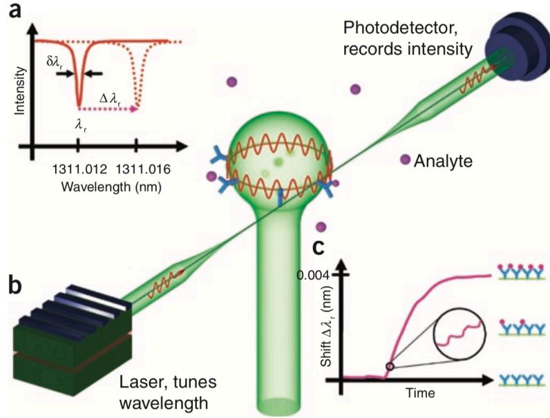
**Figure 1.** Mode-shift based sensing (a) Transmission spectra showing the mode shift. (b) Schematic of the basic WGM sensor setup. (c) Resonance wavelength shift in analyte binding process. Reproduced from ref. [42]. Copyright 2008 Springer Nature.
