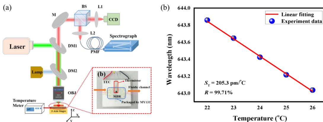
**Figure 11.** (a) The experimental setup of the WGM thermal sensor. (b) The resonance shifts as a linear function of the temperature. Reproduced from ref. <sup>[199]</sup> with permission of Multidisciplinary Digital Publishing Institute.
