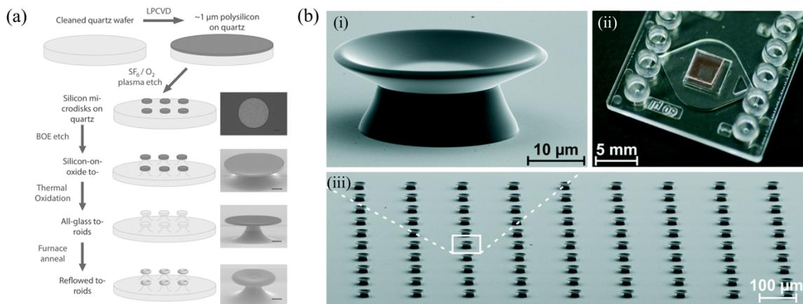
**Figure 5.** (a) Fabrication process of all-glass toroid resonators. Reproduced from ref. <sup>[118]</sup> with permission of John Wiley and Sons. (b) PMMA microgoblet lasers fabricated on a polysulfone substrate: (i) Zoom-in of a single PMMA microgoblet laser fabricated on a polysulfone substrate. (ii) Array of 100 microgoblet
