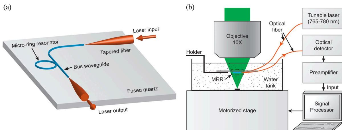
**Figure 14.** (a) Schematic illustrations of the packaged micro-ring ultrasonic detector. (b) Experimental setup of the photoacoustic microscopy system. Reproduced from ref. <sup>[224]</sup> with permission of The Optical Society.
