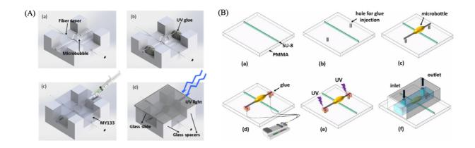
**Figure 8.** (A) Packaging process of microbubble resonators. Reproduced from ref. <sup>[166]</sup> with permission of Optical Society of America. (B) Lab-on-chip platform fabrication and packaging steps of microbottle resonators. Reproduced from ref. <sup>[167]</sup> with permission of Elsevier.
