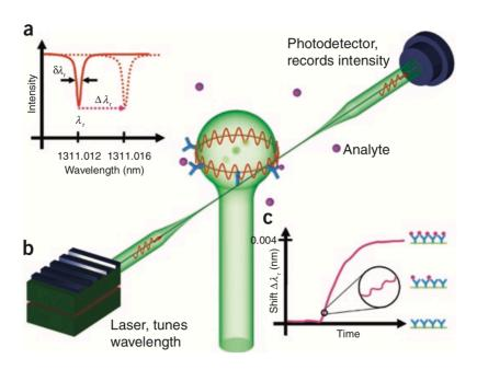
**Figure 1.** Mode-shift based sensing (a) Transmission spectra showing the mode shift. (b) Schematic of the basic WGM sensor setup. (c) Resonance wavelength shift in analyte binding process. Reproduced from ref. <sup>[42]</sup>. Copyright 2008 Springer Nature.
