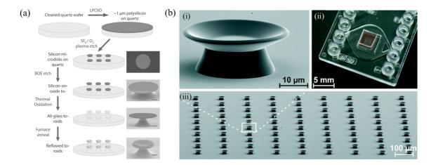
**Figure 5.** (a) Fabrication process of all-glass toroid resonators. Reproduced from ref. <sup>[118]</sup> with permission of John Wiley and Sons. (b) PMMA microgoblet lasers fabricated on a polysulfone substrate: (i) Zoom-in of a single PMMA microgoblet laser fabricated on a polysulfone substrate. (ii) Array of 100 microgoblet
