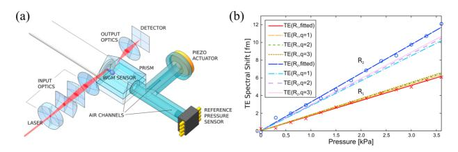
**Figure 13**. (a) Experimental setup of the WGM pressure sensing platform. (b) Spectral shift versus pressure for two spheres of radii  $R_1$ =127  $\mu$ m and  $R_2$ =89  $\mu$ m. Reproduced from ref. [213] with permission of Elsevier.
