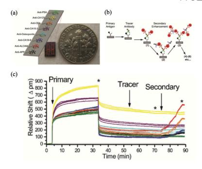
**Figure 9.** (a) Silicon microchip overlaid with four red boxes indicating sub-array regions containing 8 microring resonators, each functionalized with an antibody specific for a different cancer biomarker antigen. (b) Methodology of the layer-by-layer signal enhancement on the microring resonator silicon surface. (d) A real-time plot showing the resonance wavelength shifts through the entire bioassay. Reproduced from ref. [189] with permission of Royal Society of Chemistry.
