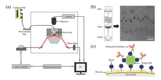
**Figure 10.** Microfluidic integrated WGMB. (a) WGMB system schematic. (b) Left: Microfluidic chip. Right: The Jurkat cells trapped in the microfluidic device. (c) Illustration of surface functionalization. Reproduced from ref. [191] with permission of John Wiley and Sons.
