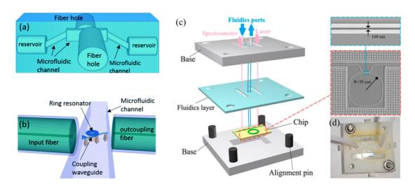
**Figure 4.** On-chip planar resonators for sensing. (a) Schematic view of the glass microfluidic chip; (b) detail of the WGM biosensor integrated inside the microfluidic channel. Reproduced from ref. [104] with permission of Royal Society of Chemistry. (c) Schematic illustration of the integrated sensing system. (d) Photograph of the PDMS microfluidic channels. Reproduced from ref. [105] with permission of AIP Publishing.
