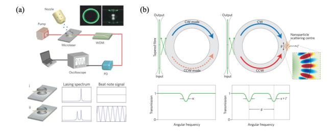
**Figure 3.** Mode-splitting sensing (a) Schematic of the experimental setup and (i) The lasing spectrum and the beat note signal before nanoparticle binding. (ii) The lasing spectrum and the beat note signal after nanoparticle binding. Reproduced from ref. <sup>[40]</sup>. Copyright 2011 Springer Nature. (b) Field distributions and transmission spectrum of mode splitting in a whispering gallery mode resonator. Reproduced from ref. <sup>[54]</sup>. Copyright 2010 Springer Nature.
