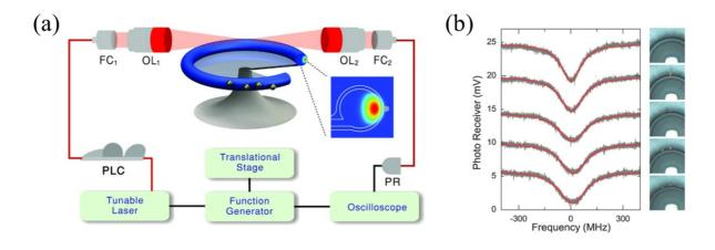
**Figure 2.** Mode-broadening based sensing (a) Experimental setup for mode-broadening based PS nanoparticles and virus detection. (b) Transmission spectra of the mode and the corresponding microcavity-enhanced-scattering optical images upon binding of 0 - 4 nanoparticles (from top to bottom). Reproduced from ref. <sup>[25]</sup>. Copyright 2013 John Wiley and Sons.
