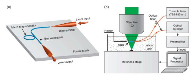
**Figure 14.** (a) Schematic illustrations of the packaged micro-ring ultrasonic detector. (b) Experimental setup of the photoacoustic microscopy system. Reproduced from ref. <sup>[224]</sup> with permission of The Optical Society.
