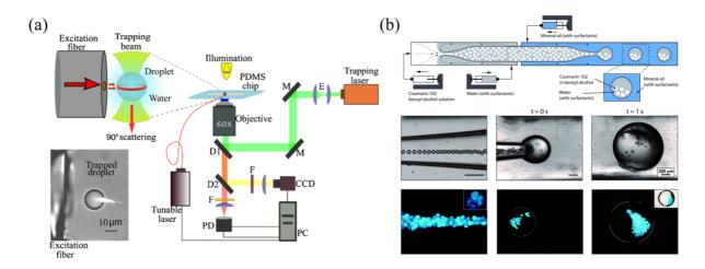
**Figure 7.** (a) Experimental setup of microdroplet scattering experiments and an image of scattered light when the trapped droplet was excited by a red laser. Reproduced from ref. <sup>[145]</sup> with permission of The Optical Society. (b) Glass capillary devices to embed liquid lasers within aqueous microfluidic droplets. Reproduced from ref. <sup>[148]</sup> with permission of Wiley Online Library.
