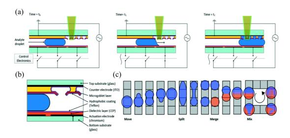
**Figure 6.** Cross-sectional view of a digital microfluidic system integrated with microgoblet resonators. (a) Analyte delivery process through activating the electrodes. (b) Close-up of the integrated system depicting the material layers (c) Some basic on-chip microfluidic operations. Reproduced from ref. [134] with permission of Royal Society of Chemistry.
