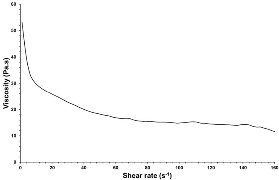
Figure 7 : Rheogramm of the robocasting tungsten paste.
