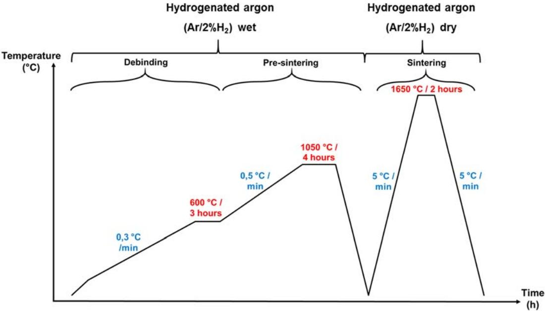
Figure 14: Thermal cycle for debinding and sintering of HTCC parts under reducing atmosphere (Ar/2%H<sub>2</sub>).
