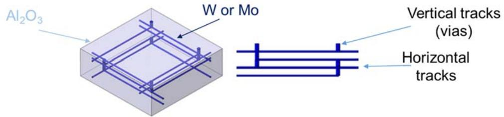
Figure 1 : Design of conventional HTCC component.
