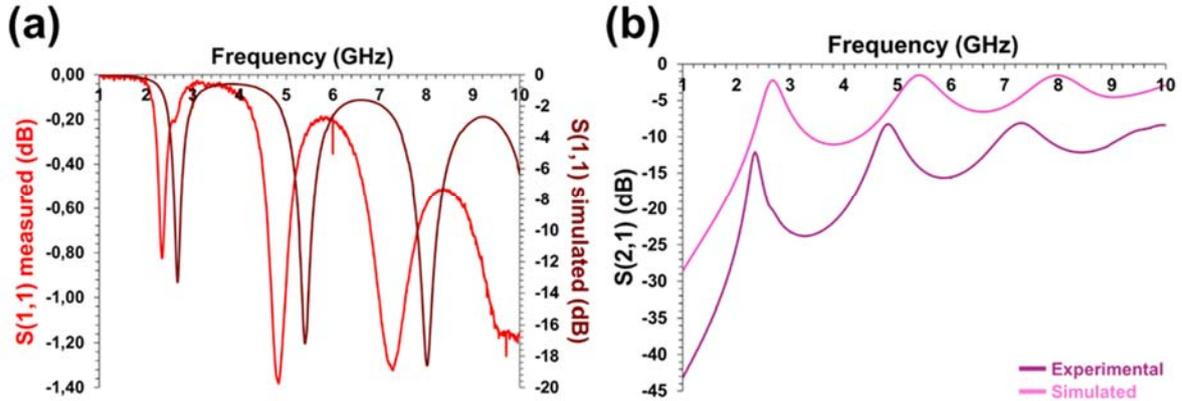
Figure 20 : Experimental frequency response curves of a HTCC embedded microstrip resonator sintered at 1650 °C for two hours under a reducing atmosphere.
