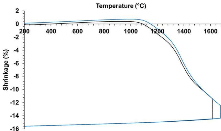
Figure 12: Dilatometry of alumina substrate at 1600 °C (black curve) and 1650 °C (blue curve) for 3h under air, 5°C/min.
