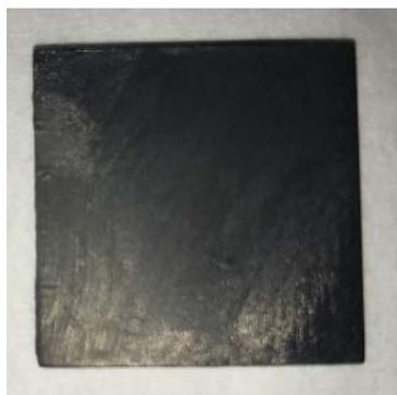
Figure 11: Alumina part obtained by stereolithography and debinded under argon at 800°C for 3 hours.
