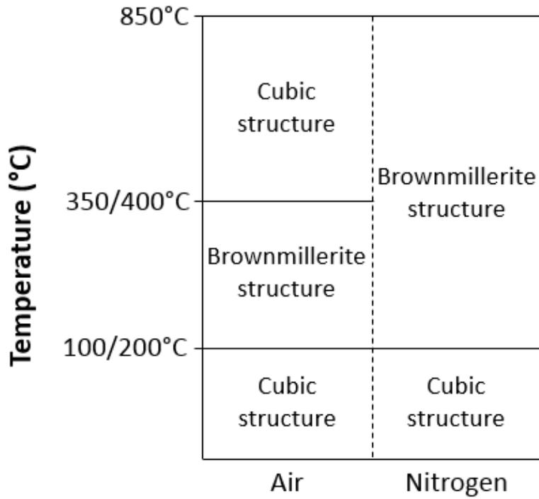
Fig. 8: Nature of the BSF73 powder structure up to 850°C under different gases
