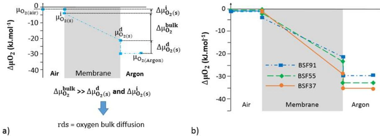
Fig. 12: Profile of the oxygen chemical potential through BSF91 perovskite membrane at  $800^{\circ}\text{C}$  with three main steps: oxygen incorporation, bulk diffusion, and desorption, b) Profiles of the oxygen chemical potential through BSF37, BSF55 and BSF91 membranes at  $800^{\circ}\text{C}$
