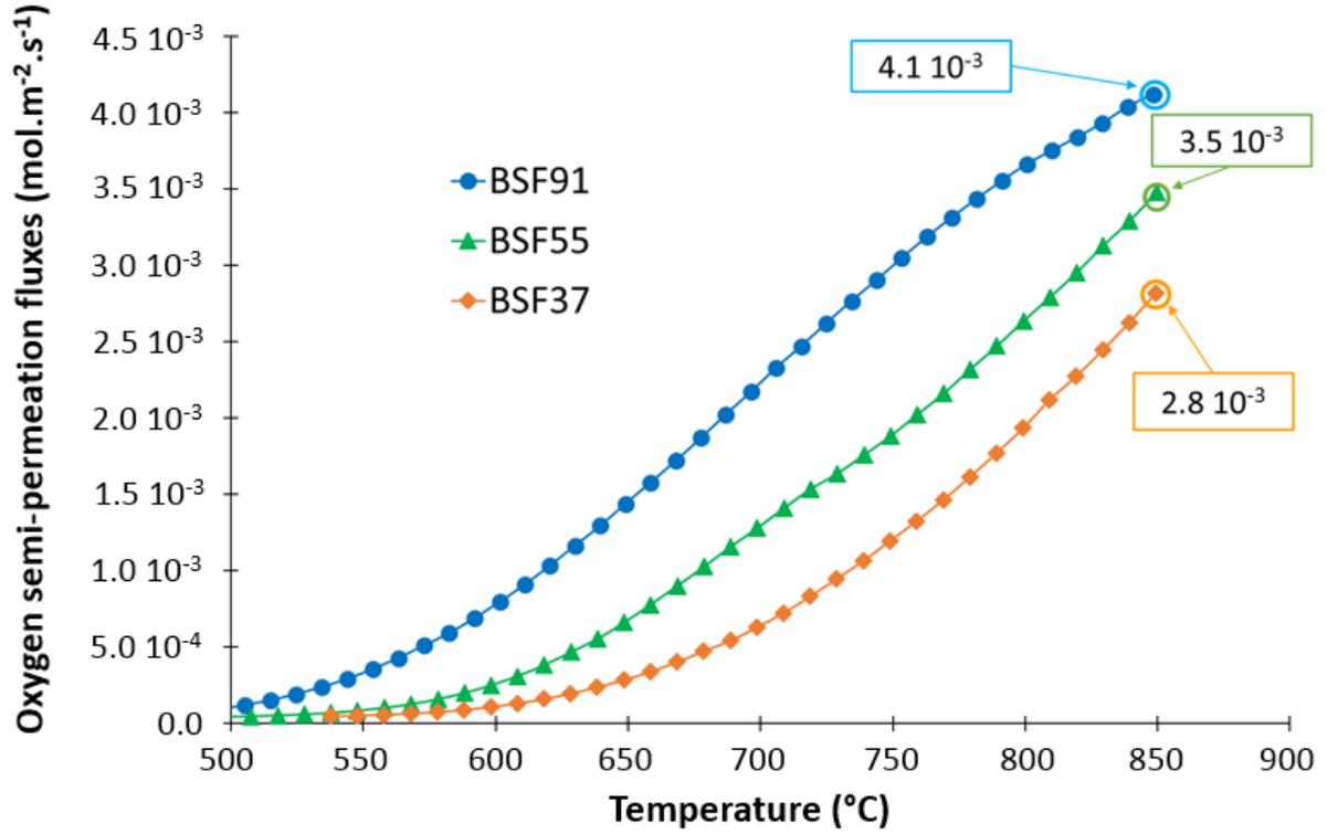
Fig. 10: Temperature dependence of the oxygen semi-permeation fluxes through dense BSF membranes under an air (100 ml.min<sup>-1</sup>)/argon (200 ml.min<sup>-1</sup>) gradient
