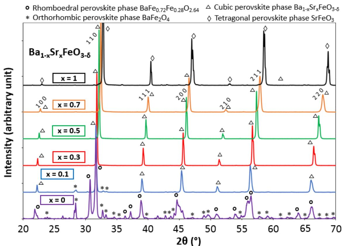
Fig. 2: X-ray diffraction patterns of  $Ba_{1-x}Sr_xFeO_{3-\delta}$  powders, with  $0 < x < 1$
