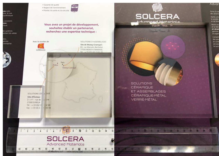
Figure 13: Example of large spinel pieces (150x150x20 mm for the largest) produced by PSC after sintering and polishing.
