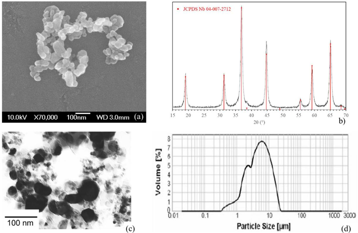
Figure 1: (a) FEG-SEM micrograph, (b) XRD pattern, (c) TEM micrograph and (d) particle size distribution of as-received spinel powder SPI-P1.
