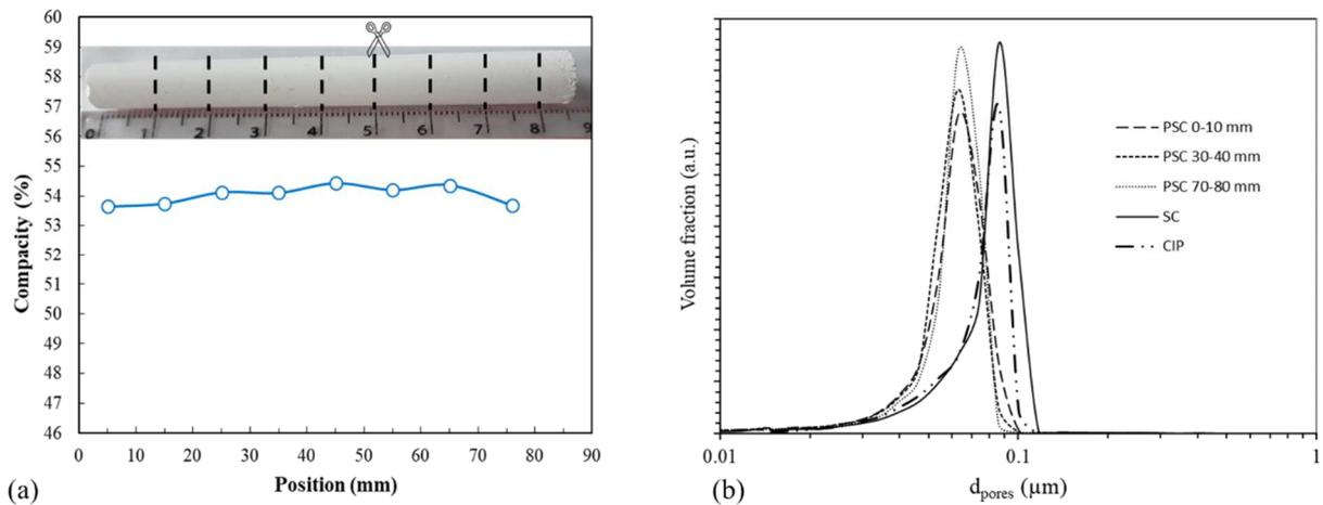
Figure 5: Compacity along a rod of YAG of 85 mm in length by 10 mm in diameter obtained by PSC (sample S5) and corresponding view (a). Comparison of the pore size distribution (Hg intrusion measurement) of YAG green compacts formed by PSC (S5a-c), SC (S3) and CIP (S6). The positions (XX-YY mm) refer to the analyzed section of the rod illustrated in (a).
