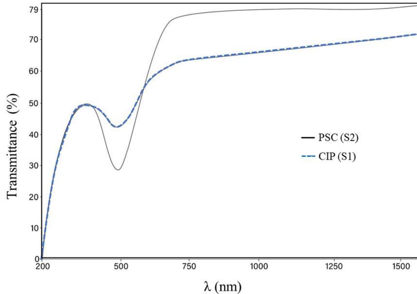
Figure 9: Transmission of YAG specimens derived from powder YAG-P1 and densified by a sinter(AS)/post-HIP approach (absorption band at 500 nm introduced by  $Y^{2+}$  see text). Top curve: green-bodies formed by PSC, lower curve: green-bodies formed by CIPing.
