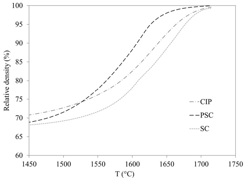
Figure 6: Relative density as a function of temperature obtained by dilatometry. Sintering was conducted under vacuum for YAG green compacts (YAG-P2) formed by PSC (**S4**), SC (**S3**) or CIP (**S6**).
