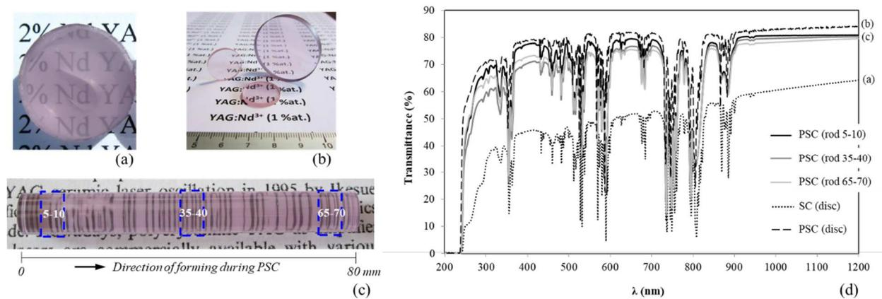
Figure 7: Pictures of 1at.%Nd:YAG ceramics from YAG-P2 powder after VS shaped by SC (**sample S3**: 25 mm in diameter, 5 mm thick) (a) or PSC in the form of discs (**sample S4**: 40 mm in diameter, 5 mm thick) (b) or rod (**sample S5**: 10 mm in diameter, 80 mm in length) (c) and corresponding optical transmission spectra (d). Analyzed zones of the rod were indicated in dotted lines with corresponding position.
