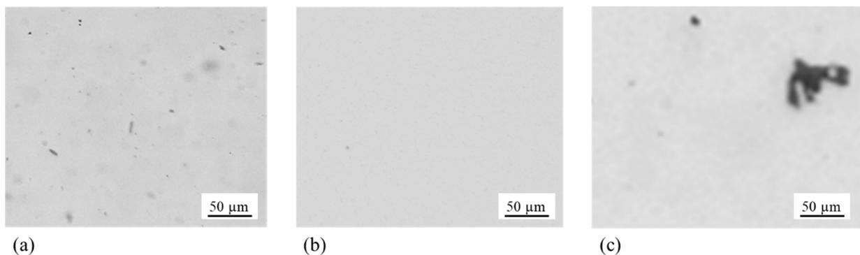
*Figure 8: Micrographs obtained by optical microscopy of 1at.%Nd:YAG ceramics from YAG-P2 powder after VS shaped by SC (**sample S3**) (a), PSC (**sample S4**) (b) or CIP (**sample S6**) (c). Residual porosity appears as black spots.*
