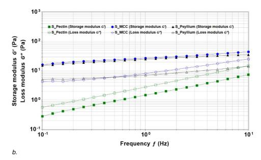
Figure 6. Stress sweep and frequency sweep measurements for S\_Pectin, S\_MCC and S\_Psyllium suspension.
