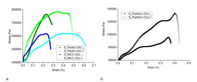
Figure 8. Stress - strain curves for the green tapes in perpendicular (Ox) and parallel (Oy) to the casting direction. a. Stress - strain curves for green tapes obtained with the suspensions S\_Pectin and S\_MCC; b. Stress - strain curves for green tapes obtained with the suspension S\_Psyllium in perpendicular (Ox) and parallel (Oy) to the casting direction
