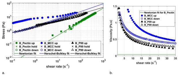
Figure 2. Rheological behavior of the three binder systems at 22°C. The stress was raised from 0.01 to 20 Pa for 60 s, followed by a peak hold at 20 Pa during 60 s, and finally a decrease from 20 to 0.01. Pa in 60 s. The relevant fits for each decreasing ramp are also shown. a. Stress as a function of shear rate. b. viscosity as a function of shear rate, zoom below 31 s<sup>-1</sup>.
