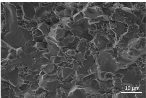
**a)** Microstructure of green dried alumina tape based on S\_Pectin suspension (citrus pectin)
