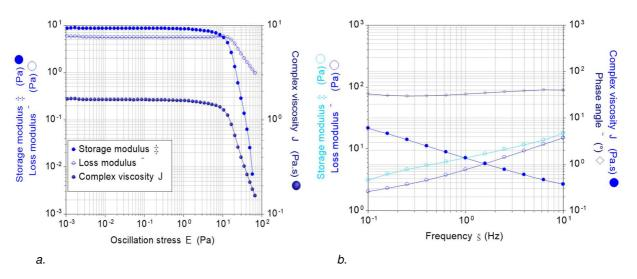
Figure 3: MCC rheological oscillatory behavior (a: evolution of the storage modulus and of the viscosity as a function of the stress, f = 1 Hz; b: evolution of the storage and the loss modulus and of the viscosity and the phase angle as a function of the frequency as a function of frequency,  $\sigma = 10^{-2}$  Pa)
