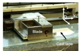
Figure 7. Photograph of the casting of a tape. Indications of the considered directions.
