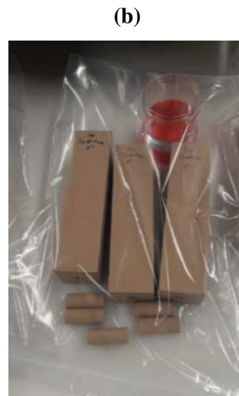
Figure 3. Photo (a) of the shrinkage measurement and (b) of the sample storage in sealable plastic bag
