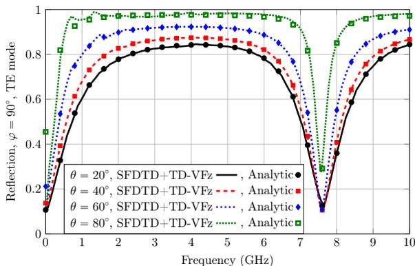
Fig. 5: Reflection coefficient magnitude for the two layers.
