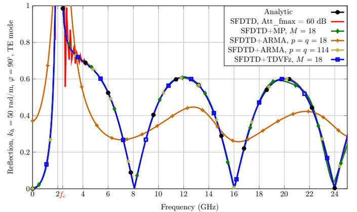
Fig. 2: Reflection coefficient for the homogeneous layer.
