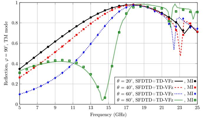
Fig. 7: Reflection coefficient magnitude for the JCFSS.
