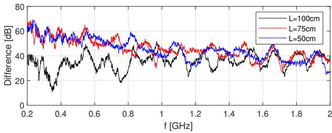
Fig. 8. Comparison of the average difference of magnitude of the  $S_{21}$  parameter for the unshielded and the shielded TWP over all the mode stirrer positions in the unloaded RC for 3 different lengths of the TWPs.
