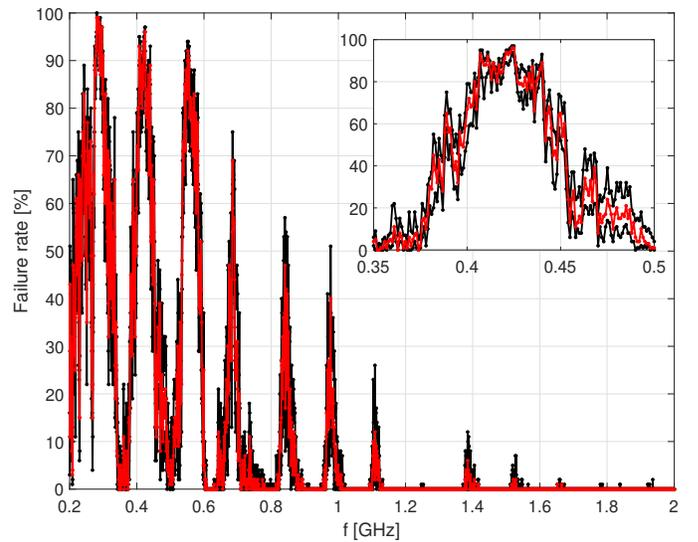
Fig. 10. Failure rate obtained on the unshielded TWP of 1 m length for the unloaded RC and for the first position of the emitting antenna (for  $\langle |E_T| \rangle = 100$  V/m and  $\tau = 0$  dB). The red plot corresponds to the results obtained for  $\langle |E_T| \rangle = 100$  V/m while black plots are related to  $\langle |E_T^{min}| \rangle$  and  $\langle |E_T^{max}| \rangle$ . The inset is a zoom between 0.35 and 0.5 GHz.
