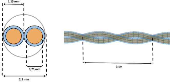
Fig. 4. Schematic description of the cross-section geometry of the unshielded TWP (on the left) and of its longitudinal view (on the right). Note that only 1 TWP is represented.
