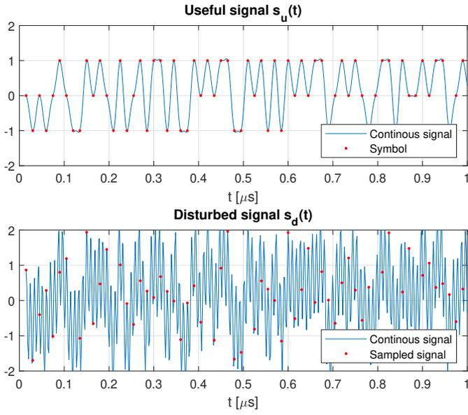
Fig. 17. Time-domain waveform (over  $1 \mu\text{s}$ ) of the useful 100BASE-T1 signal  $s_u(t)$  and of the disturbed signal  $s_d(t)$ . The parasitic signal is the sum of 2 harmonic disturbances of 300 and 370 MHz calculated from the maximum value of  $V_{dm}$  in the case of the unshielded TWP of length 90 cm (for  $\langle |E_T| \rangle$  of 100 V/m).
