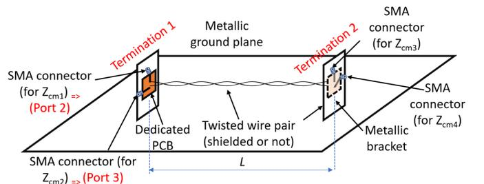
Fig. 2. Schematic description of the cable under test.
