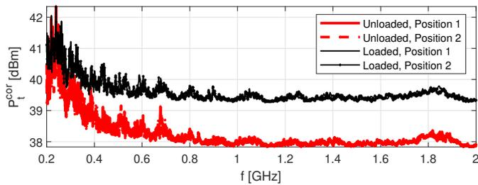
Fig. 11. Comparison of the transmitted power  $P_t^{cor}$  required to obtain  $\langle |E_T| \rangle = 100 \text{ V/m}$  in the RC for both positions of the emitting antenna and both loading conditions.
