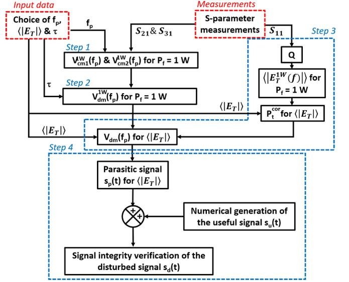
Fig. 5. Flowchart presenting the different steps of the method. This process can be repeated for each set of input data (i.e.  $f_p$ ,  $I_{bc}$  and  $\tau$ ) of the parasitic signal  $s_p(t)$  and for each stirring configuration (i.e. each mode stirrer position for a mechanically stirred RC).
