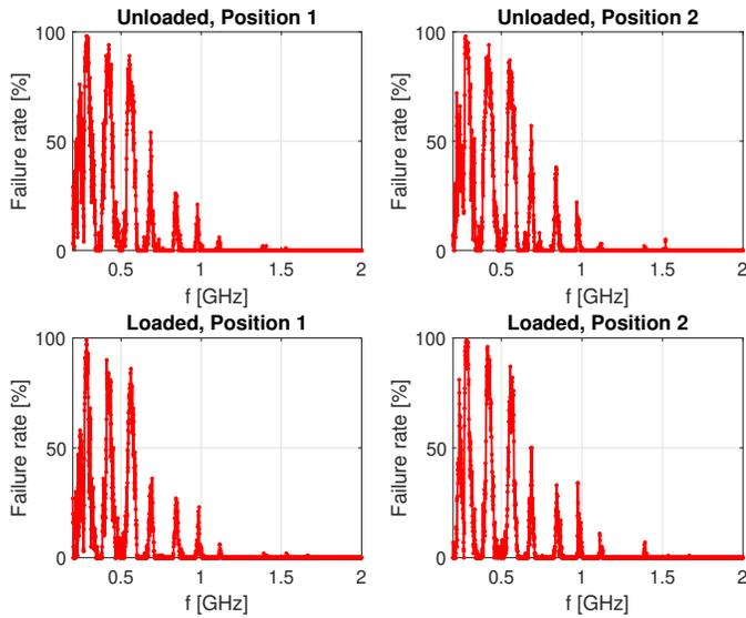
Fig. 12. Failure rate obtained on the unshielded TWP of 1 m length for two different positions of the antenna and both loading conditions (for  $\langle |E_T| \rangle = 100 \text{ V/m}$  and  $\tau = 0 \text{ dB}$ ).
