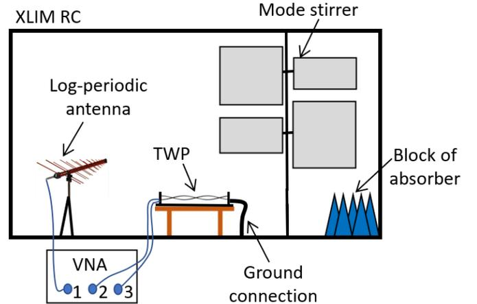
Fig. 1. Schematic description of the required measurement setup. A 2-port VNA is also usable after modifying the successive ports to measure and inserting a  $50 \Omega$  impedance on each unconnected port. The presence of the block of absorber is optional.
