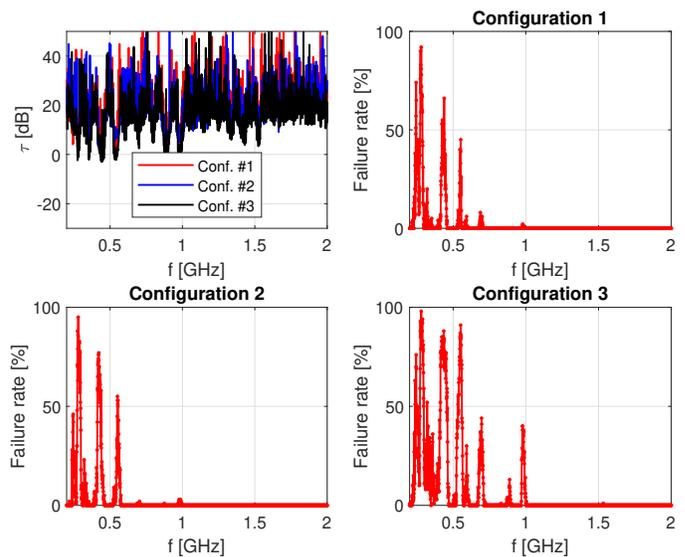
Fig. 13. Comparison of the common-mode rejection rate  $\tau$  (top, left) and failure rate obtained on the unshielded TWP of 1 m length in the unloaded RC for the three common-mode impedance configuration described in Table I (for  $\langle |E_T| \rangle = 100 \text{ V/m}$ ).
