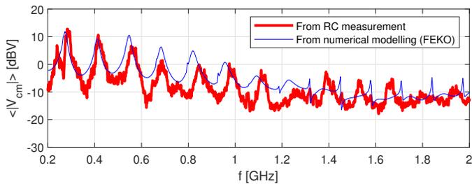
Fig. 15. Comparison of the CM voltage obtained on a  $50 \Omega$  load in a balanced configuration from RC measurements and in Simulations (FEKO) for  $\langle |E_T| \rangle$  of 100 V/m on an unshielded TWP of 1 m length.
