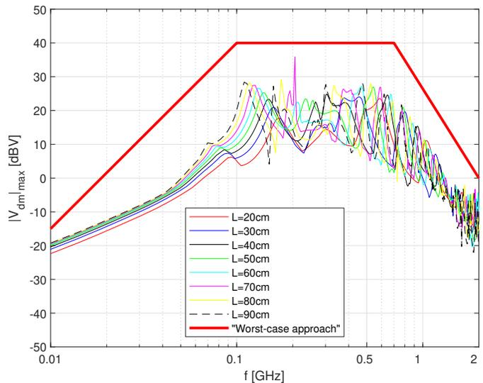
Fig. 16. Comparison (from FEKO simulations) of the maximum DM voltage obtained for all the plane wave spectrum in the unbalanced configuration on 8 unshielded TWPs of different lengths (for  $\langle |E_T| \rangle$  of 100 V/m). The thick line could correspond to the level considered in the case of a typical EMC study based on a “worst-case approach” guaranteeing a safety margin of a few dB.
