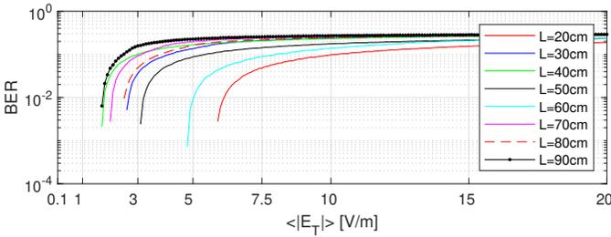
Fig. 18. Bit-error-rate (BER) as the function of  $\langle |E_T| \rangle$  obtained on the 100BASE-T1 signal from numerical simulations on unshielded TWPs of different lengths. The computation is made on the maximum value of  $V_{dm}$  calculated at each frequency over the 50 simulations. The parasitic signal is the sum of 2 harmonic disturbances of 300 and 370 MHz.
