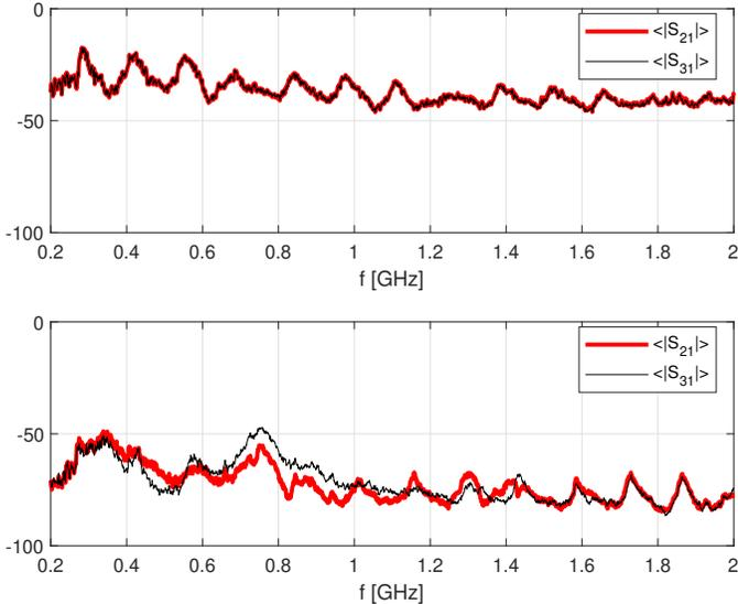
Fig. 9. Comparison of the average magnitude of  $S_{21}$  and  $S_{31}$  (expressed in dB) over all the mode stirrer positions in the unloaded RC for the unshielded TWP (top subplot) and the shielded one (bottom subplot).
