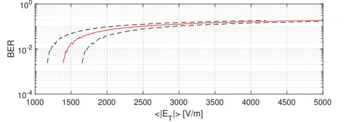
Fig. 20. Bit-error-rate (BER) as the function of  $\langle |E_T| \rangle$  obtained on the 100BASE-T1 signal from numerical simulations on the shielded TWP of 50 cm length. The computation is made on the maximum value of  $V_{dm}$  calculated at each frequency over the 50 simulations. The parasitic signal is the sum of 2 harmonic disturbances of 300 and 370 MHz. The BER is also plotted for an uncertainty on  $\langle |E_T| \rangle$  of  $\pm 1.5$  dB (dashed line).
