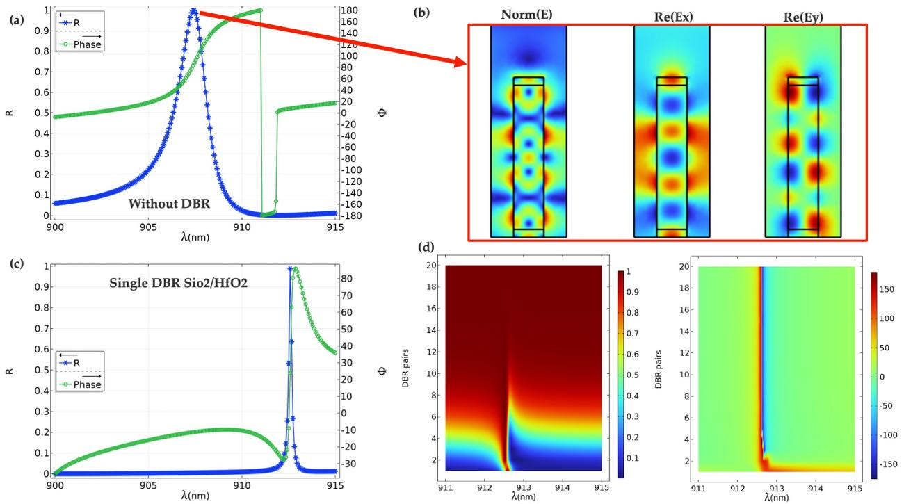
**Figure 7** Results of the unit cell for the MQW configuration in Fig. 4. (a) For the amplitude and phase response of the structure without DBR (the single resonator is surrounded by air from above and below). The corresponding field profiles at resonant frequency are given in (b). (c) Amplitude and reflection phase response for a resonator placed on a single DBR pair of SiO<sub>2</sub>/HfO<sub>2</sub>. (d) for the evolution of amplitude and phase as a function of DBR pairs.
