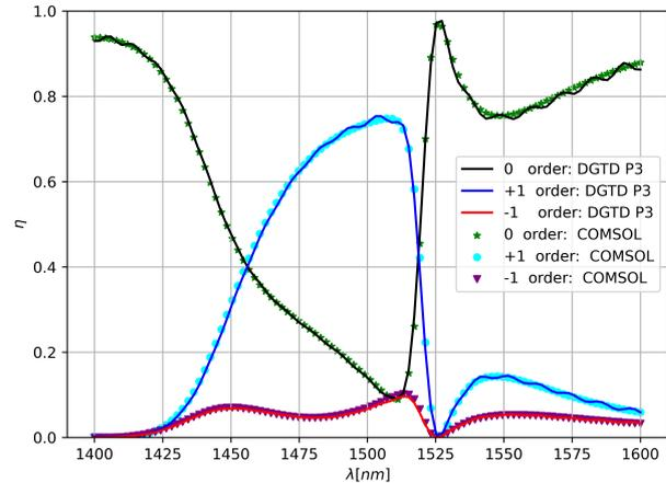
**Figure 5** Comparison between results obtained for an active thermal beam steering configuration (see Fig. 3 for more details) using the DG solver developed in our DIOGENeS [71] (lines) and results obtained using the commercial COMSOL Multiphysics® v. 6.0 software (points) based on the FEM methodology. The refractive index distribution have unexpected spatial variation as indicated in the second column of the table. 1.
