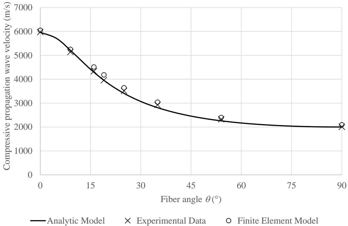
Fig. 12 Evolution in numerical VP vs. the fiber angle
