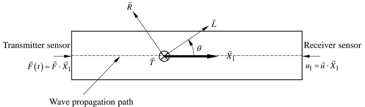
Fig. 11 Compression wave propagation diagram
