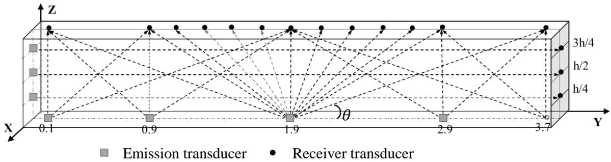
Fig. 2 Ultrasonic transducer locations for measuring wave velocity vs. angle range
