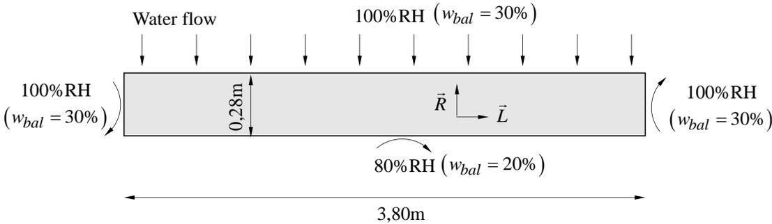
Fig. 13 Convective conditions in the moisture uptake
