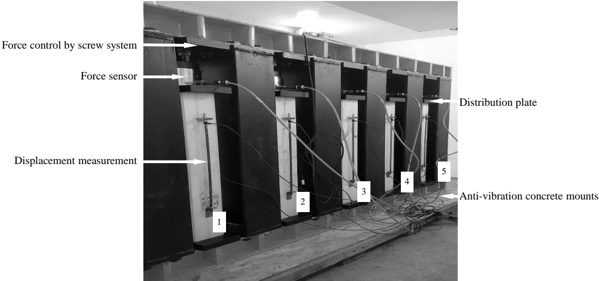
Fig. 3 Experimental creep device
