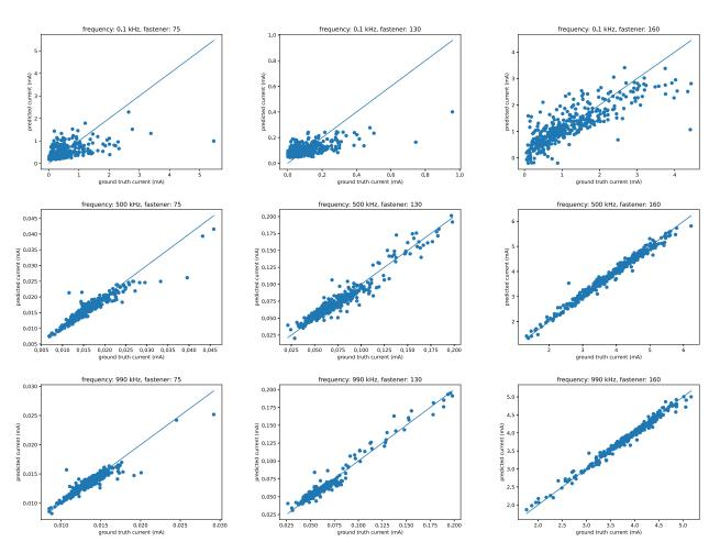
Fig. 10. Predicted values versus ground truth for fasteners 75 (left), 130 (middle), 160 (right), and for frequencies 100 Hz (top), 500 kHz (middle), 990 kHz (bottom). The line corresponds to perfect predictions.
