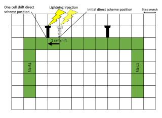
Fig. 4. Illustration of the direct scheme with one cell shift.
