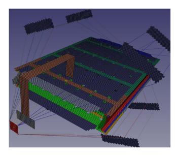
Fig. 3. Fuel tank FDTD mesh in an attachment mode [9].
