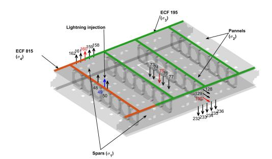
Fig. 8. Illustration of the main parameters around the observation points (in red).
