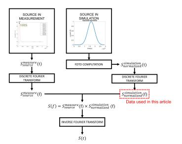
Fig. 5. Flowchart of the post-treatment used in [9].
