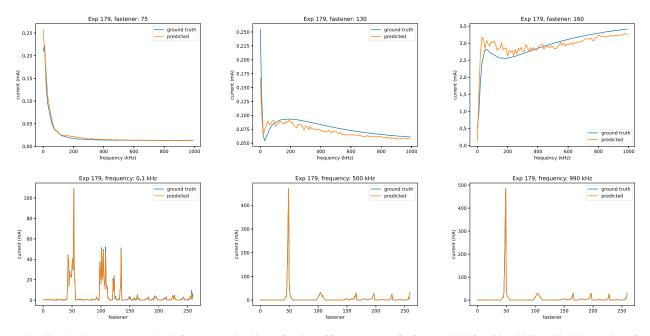
Fig. 11. Predicted value versus ground truth for test sample 179 as a function of frequency (top) for fastener 75 (left), 130 (middle), 160 (right), and as a function of position (bottom) for frequency 100 Hz (left), 500 kHz (middle), 990 kHz (right).
