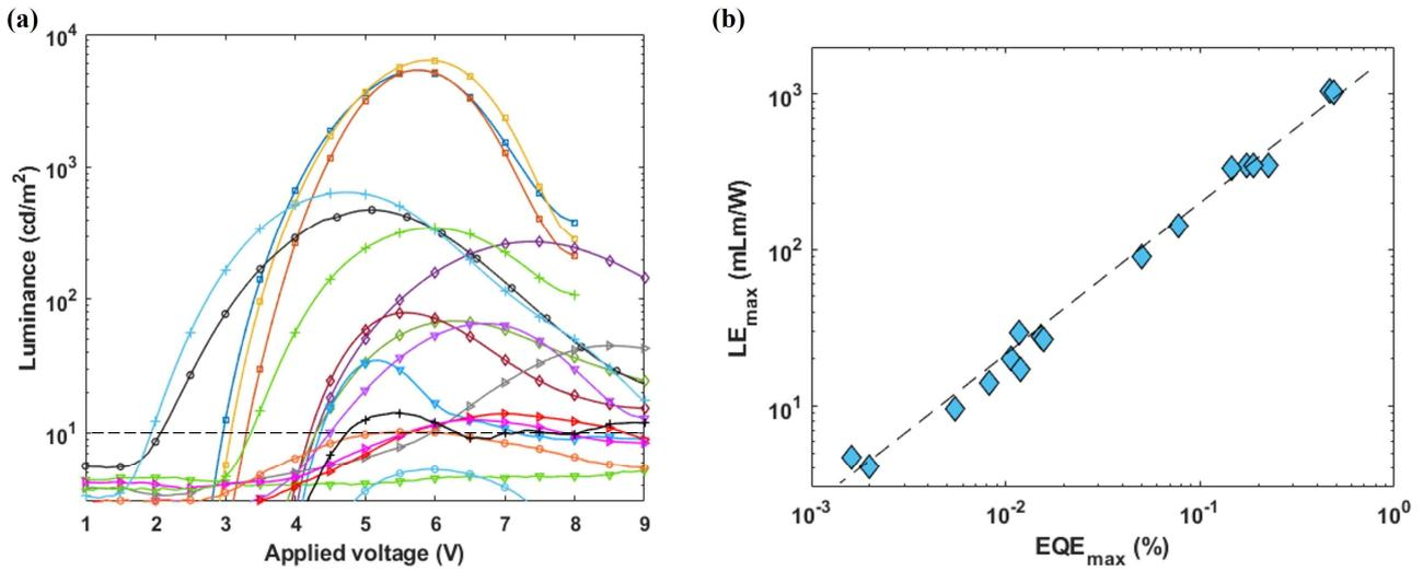
**Figure 1.** Device performance measured from a set of 17 quasi-2D perovskite LEDs prepared from the standard Set-up A configuration: (a) luminance–voltage curves (each color is a different device from the same batch), where the dotted line indicates the threshold luminance of 10 cd/m<sup>2</sup> and (b) dispersion of maximum EQE and LE values for the device set. The straight line represents the linear relation between the two quantities.
