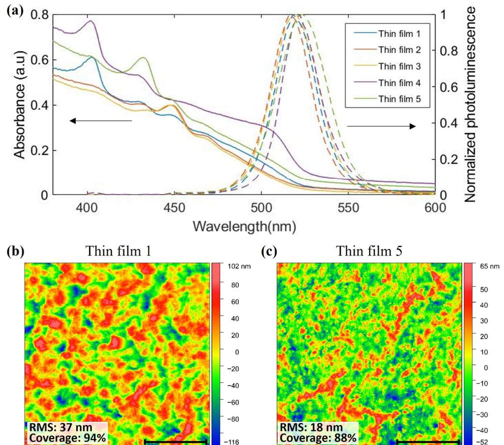
**Figure 2.** (a) UV–visible absorption (solid lines) and steady-state PL spectra (dotted lines) of intrabatch perovskite thin films deposited successively using Set-up A; (b,c) AFM images of the first and the last samples in the batch. The scale bar is 10 µm.
