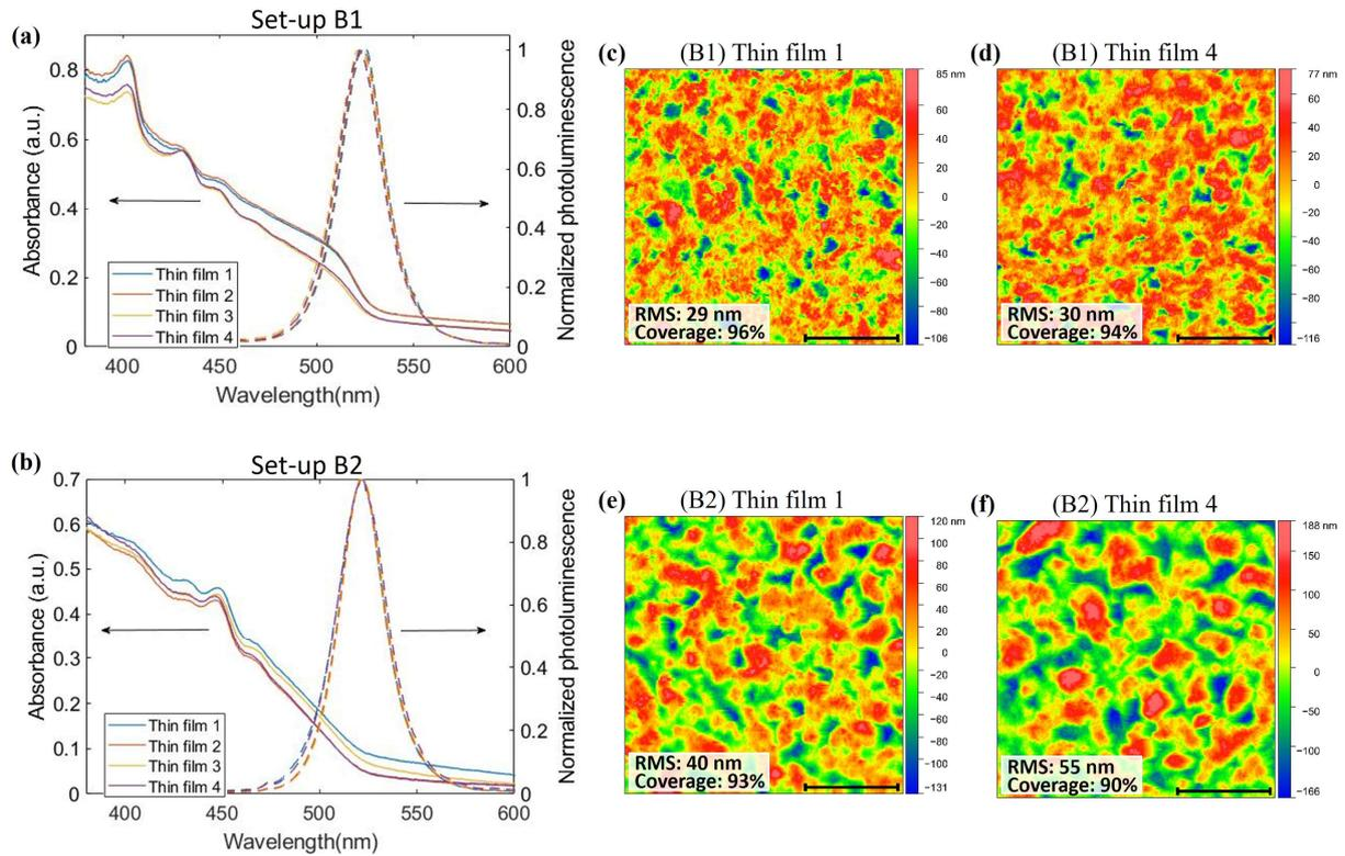
**Figure 3.** (a,b) Absorption (solid lines) and steady-state PL spectra (dotted lines) of intrabatch perovskite samples deposited successively using Set-ups B1 and B2; AFM images of the first and the last samples in the batch with respect to (c,d) Set-up B1 and (e,f) Set-up B2. The scale bar is 10  $\mu\text{m}$ .
