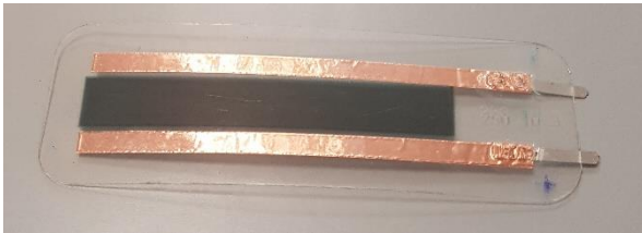
FIGURE 4. OPV based on LAYER® technology. Fabricated by Dracula Technologies.
