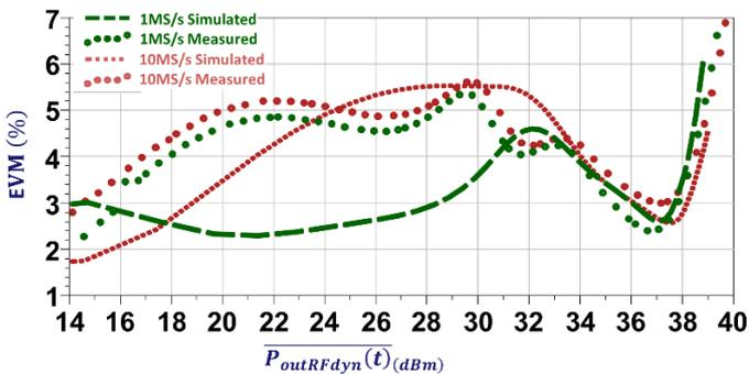
Fig. 9. Simulated and Measured Power performances of the DPA ( EVM vs  $\overline{P_{outRFdyn}(t)}$ ) driven with the 16-QAM 10 MS/s modulated signal.
