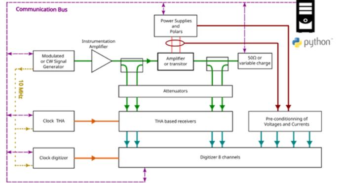
Fig. 5. 8-channel time-domain measurement system for power measurements of non-linear devices, driven by the CW signal and injected in the  $\pi_{inDPA}$  plane.
