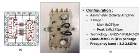
Fig. 1. Layout (a), Demonstration board (b) and Key Characteristics (c) of the realized asymmetric packaged Quasi-MMIC SI-DPA [2].
