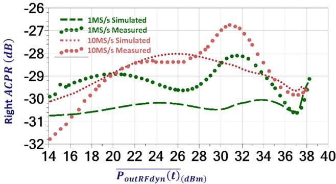
Fig. 8. Simulated and Measured Power performances of the DPA ( Right ACPR vs  $\overline{P_{outRFdyn}(t)}$ ) driven with the 16-QAM 10 MS/s modulated signal.
