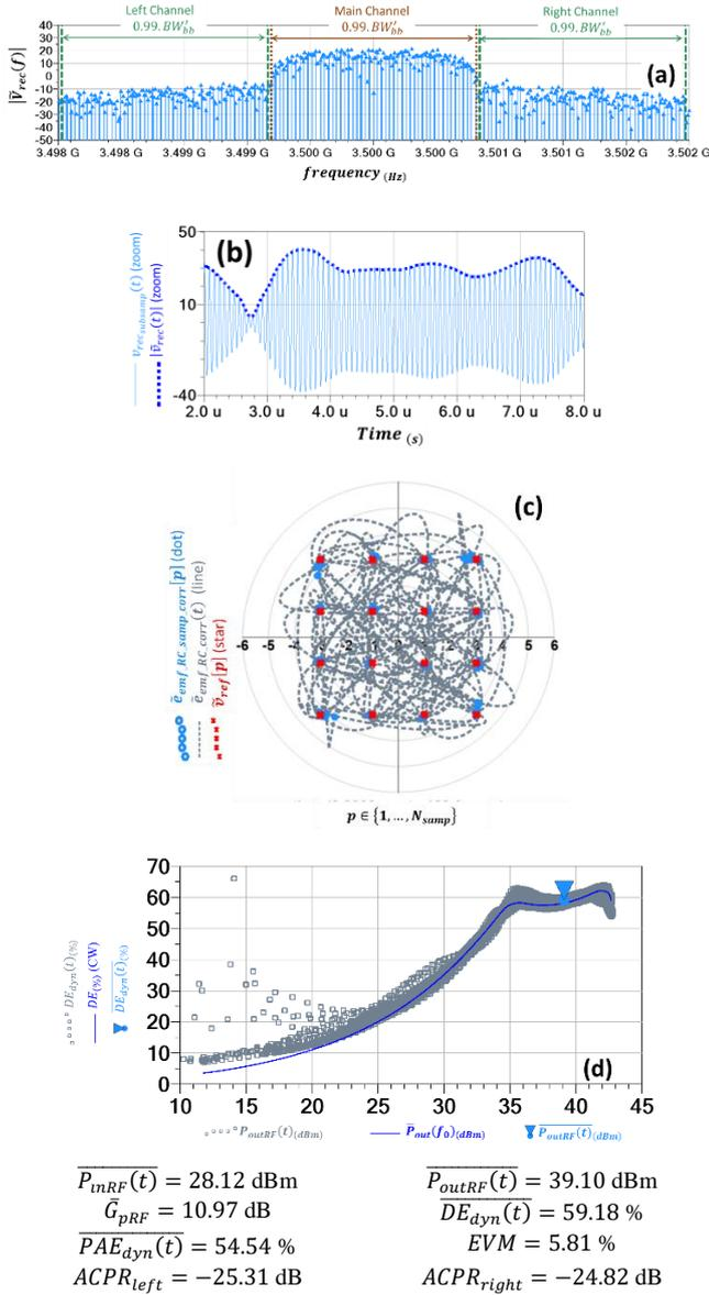
Fig. 4. Main results of the PRM-HB simulation of the DPA driven by the modulated 16-QAM EMF for  $A_{car} = 5.15V$  and for  $S_{ymbRate1} = 10MHz$ .
