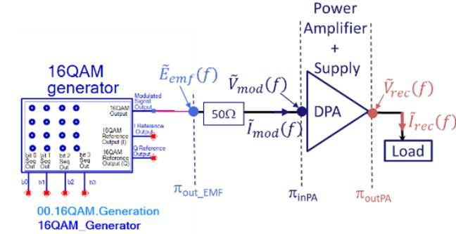
Fig. 2. Definitions of the frequency-domain variables for calculation of the modulated power performances.
