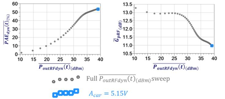
Fig. 3. Results of the PRM-HB simulation of the DPA driven by the modulated 16-QAM:  $PAE_{dyn}(\%)$  versus  $P_{outRFdyn}(t)(dBm)$  (Left) and  $PAE_{dyn}(\%)$  versus  $P_{outRFdyn}(t)(dBm)$  (Right) with indication of the selected samples for  $A_{car}=5.15V$  and for  $S_{ymbRate1} = 1\text{MHz}$ .
