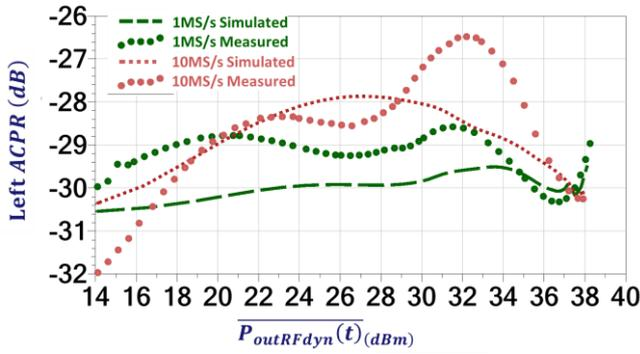
Fig. 7. Simulated/Measured Left ACPR vs  $\overline{P_{outRFdyn}(t)}$  of the DPA driven with the 16-QAM 10 MS/s modulated signal at 1MS/s and 10MS/s.
